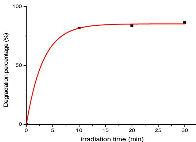
**Figure (3.3) The relation between the exposure time and the degradation percentage of a mixture composed of 5 ml Malachite green and 300 mg CuO.**
