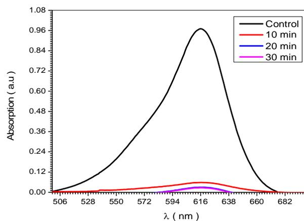
**Figure (3.4): The absorption spectra of Malachite green mixed with 500 mg of CuO irradiated by UV light for different exposure times.**
