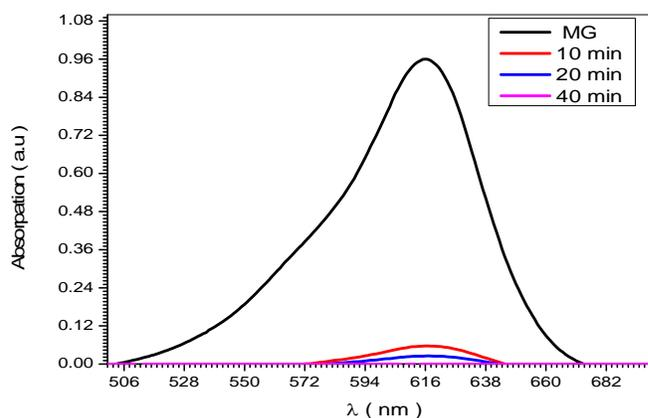
**Figure (3.6): The absorption spectra of Malachite green mixed with 1000 mg of CuO irradiated by UV light for different exposure times**
