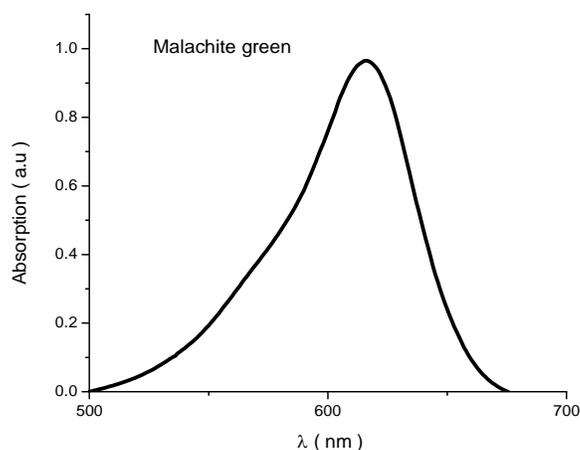
**Figure (3.1): the absorption spectrum of malachite green in 100 ml distilled water without irradiation and without semiconductor**
