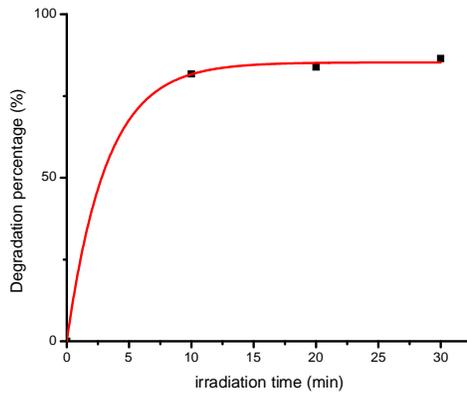
**Figure (3.5) The relation between the exposure time and the degradation percentage of a mixture composed of 5 ml malachite green and 500 mg CuO.**
