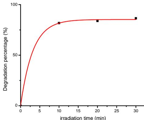
**Figure (3.7) The relation between the exposure time and the degradation percentage of a mixture composed of 5 ml malachite green and 1000 mg CuO.**
