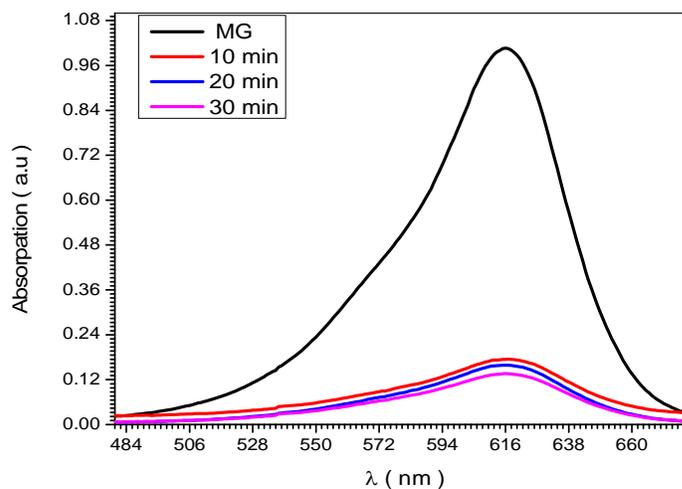
**Figure (3.2):** The absorption spectra of Malachite green mixed with 300 mg of CuO irradiated by UV light for different exposure times.
