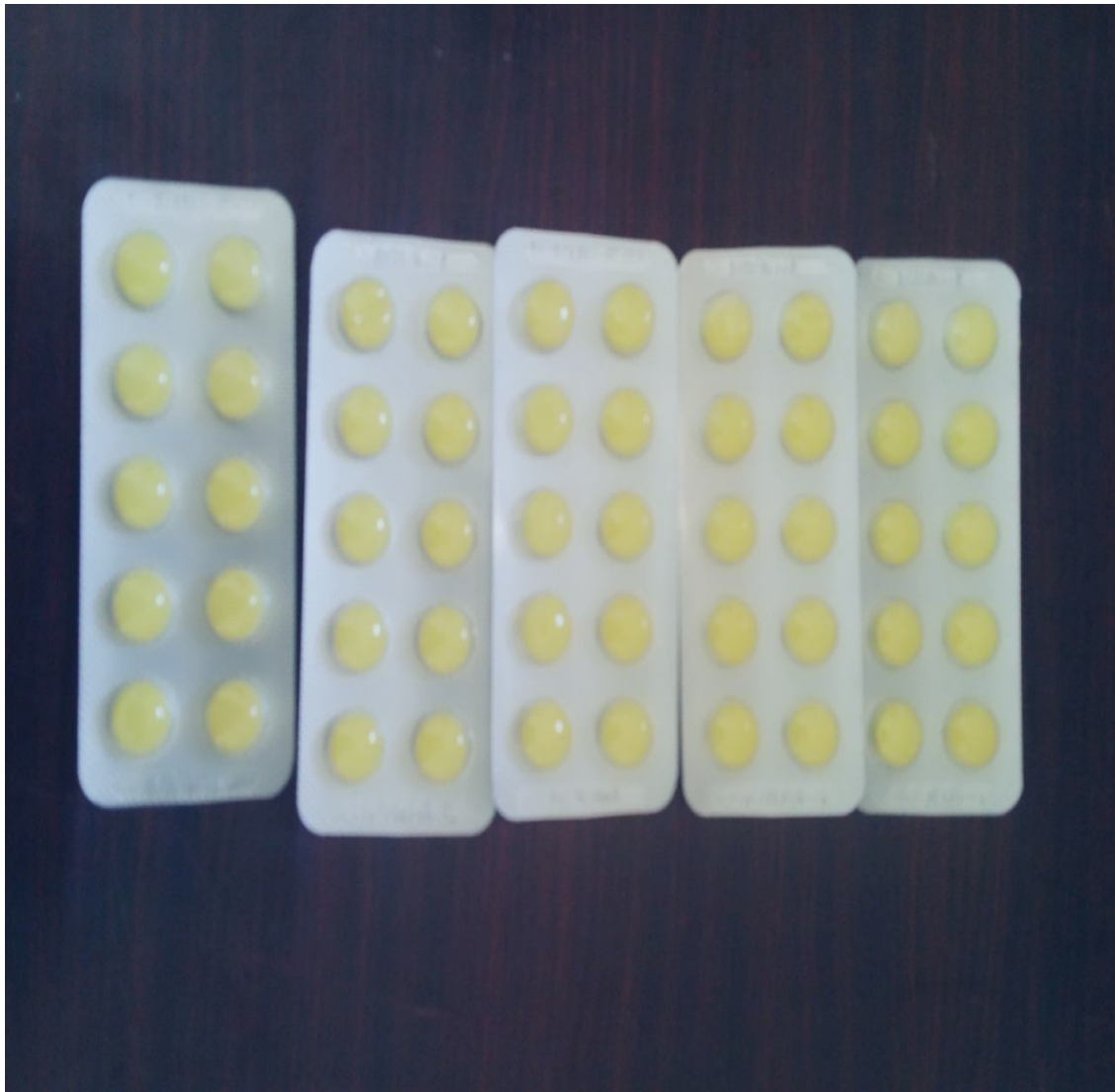
Figure 20: Metronidazole Tablet after Blistering
