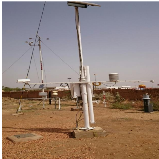
Figure2-13: VISALA automatic station
