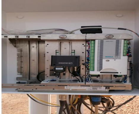
Figure 2-12: AWS box containing battery and GSM module
