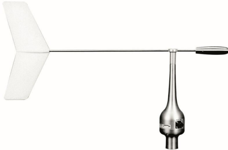
Figure 2-10: a tail vane used to measure wind direction
