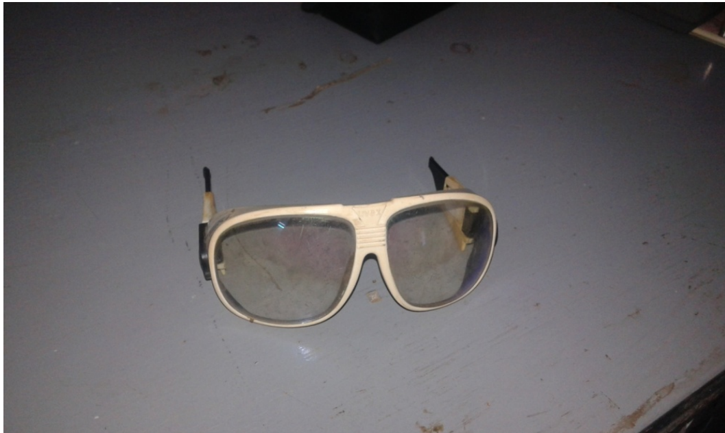
Figure 3.1. Goggle with wavelength (1064-1048) nm
