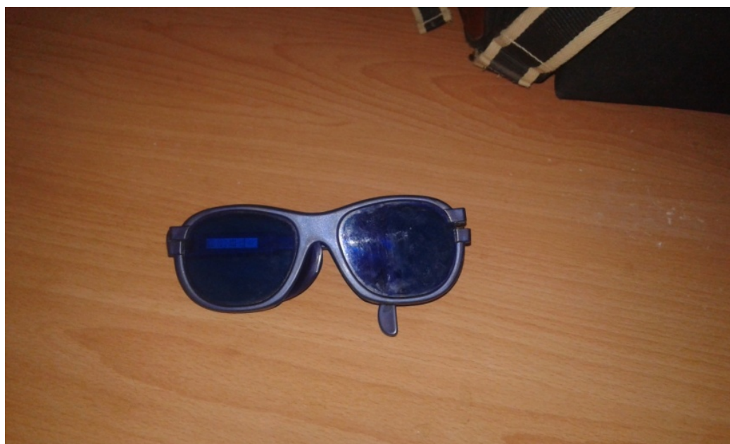
Figure 3.3. Goggle with wavelength (870-694and 830-904) nm
