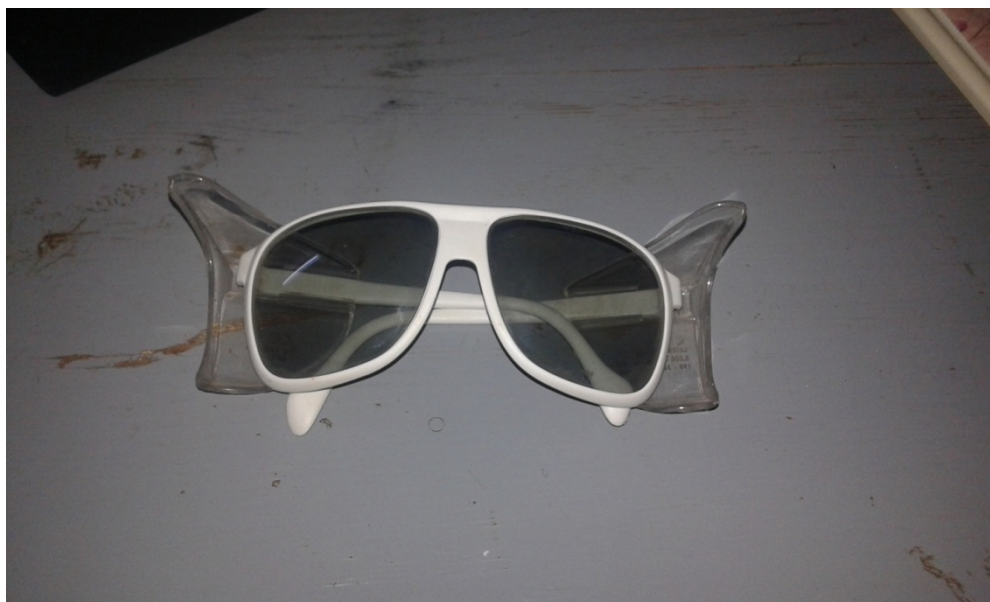
Figure 3.4. Goggle with wavelength (190-380 and 5000-11000) nm
