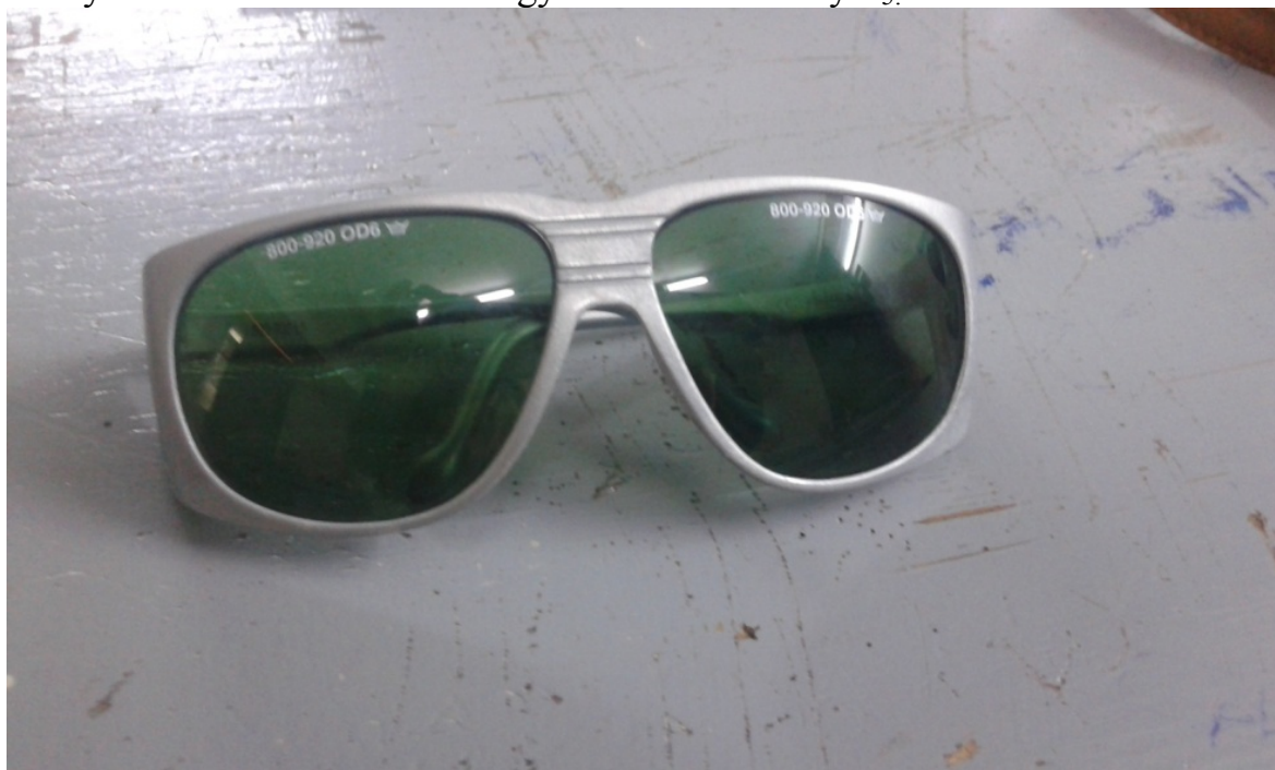
Figure 3.5. Goggle with wavelength 800-920 nm
