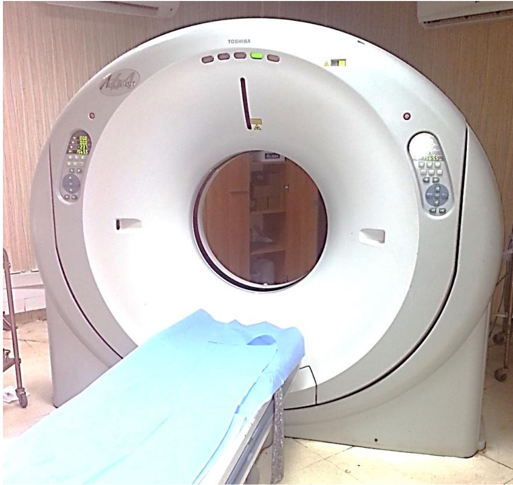
Figure (3-2) Toshiba Aquilion™ 64 CFX CT scanner ,Gantry and Table. Royal Scan, CT Department, Khartoum 2015
