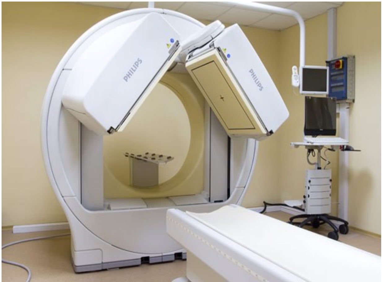
Figure (3-2) BrightView SPECT is variable angle gamma camera. This is the camera used for imaging patients.
