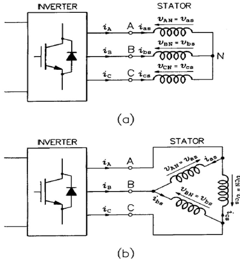
FIGURE 5.2 Stator currents and voltages: (a) wye-connected stator, (b) delta connected stator.
