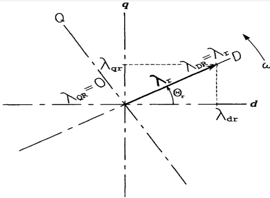
FIGURE 5.6: Alignment of the revolving reference frame with the rotor flux vector.
