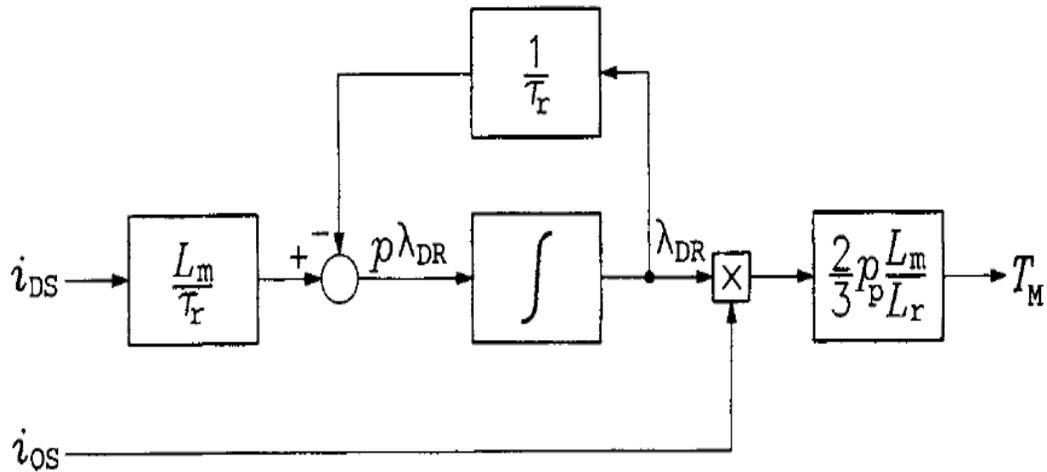
FIGURE 5.7 Block diagram of the field-oriented motor in a revolving reference frame aligned with the rotor flux vector.
