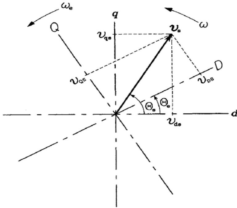
FIGURE 5.4 Space vector of stator voltage in the stationary and revolving reference frames.
