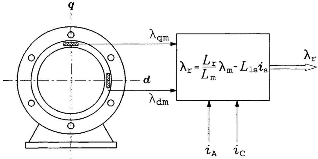
FIGURE 5.9 Estimation of the rotor flux vector based on direct measurements of the air-gap flux.
