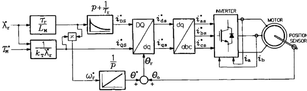
FIGURE 5.11 Block diagram of the ASD with indirect rotor flux orientation.
