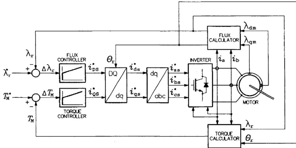
FIGURE 5.10: Block diagram of the ASD with direct rotor flux orientation.
