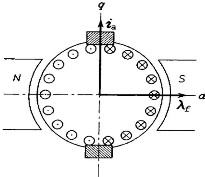
FIGURE 5.5 Simplified representation of the dc motor.
