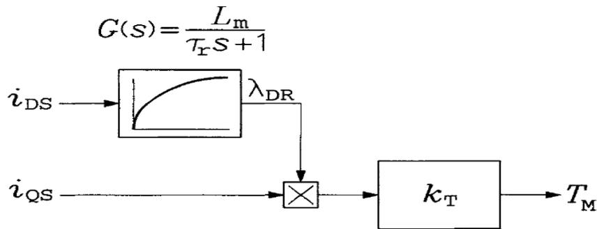
FIGURE 4.8: Reduced block diagram of the field-oriented motor in a revolving reference frame aligned with the rotor flux vector.
