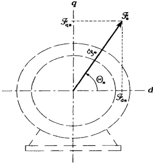
FIGURE 5.1 Space vector of stator MMF.
