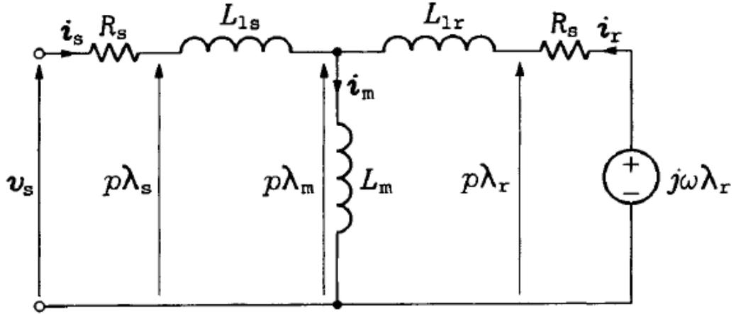
FIGURE 5.3 Dynamic T-model of the induction motor.
