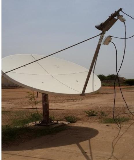
Figure 4.12 : 2.4 m Remote Antenna
