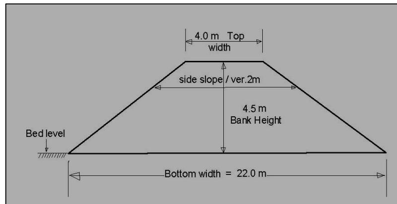
**Fig.(5.20):Cross Section Of Outer Guide Bank**
