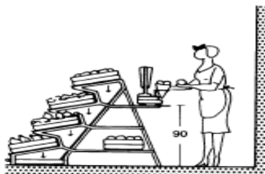
8 Counter with stands for boxes and baskets, drip pan and dirt trap
