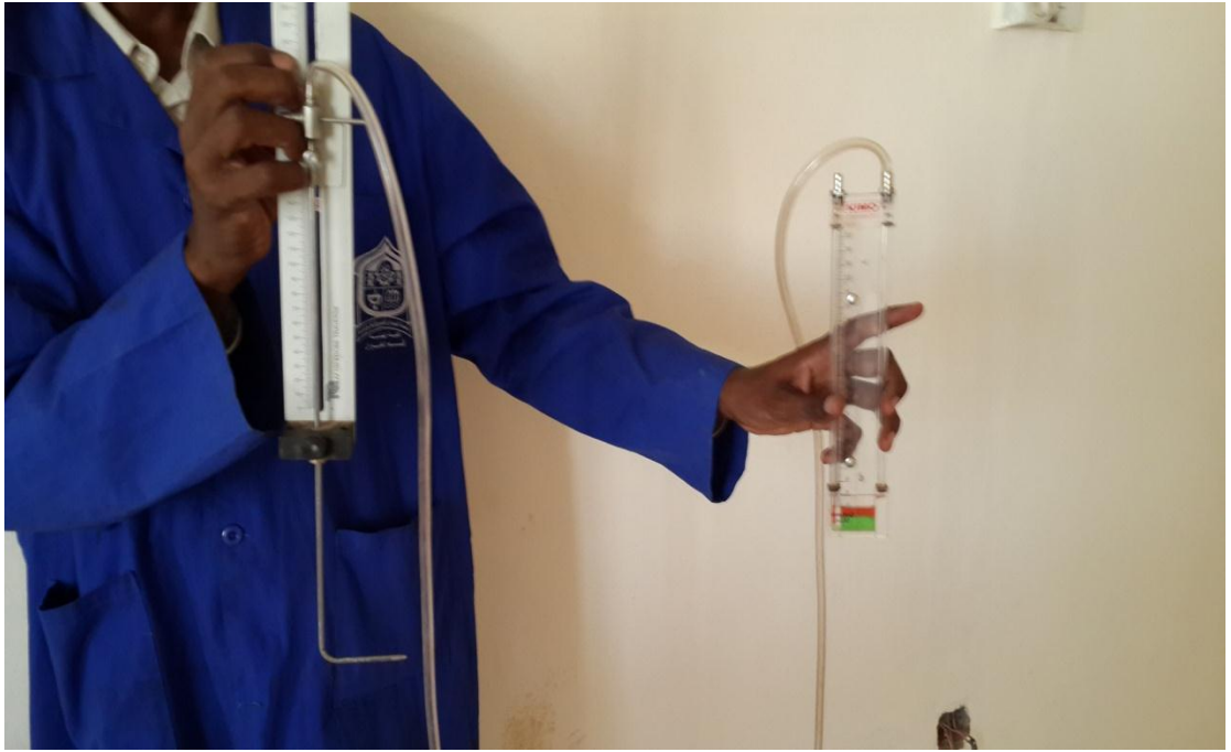
Figure 7-10: Pitot-tube and the manometer
