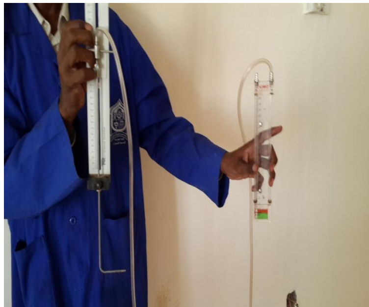
Figure 8-12: Pitot tube with manometer
