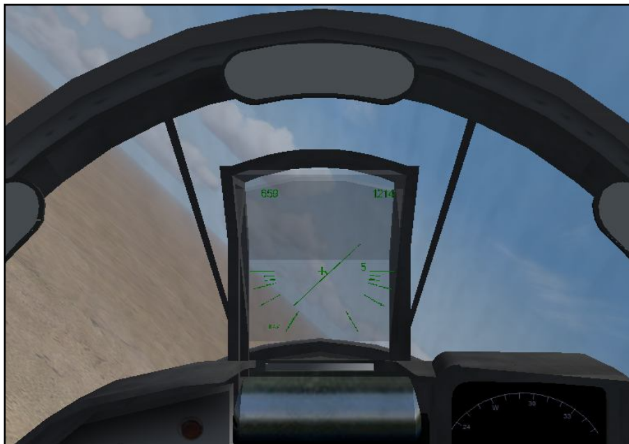
Figure (4.2-c): Virtual-cockpit view: puts the pilot's eyes inside a three-dimensional aircraft's cockpit with ability to look around.
