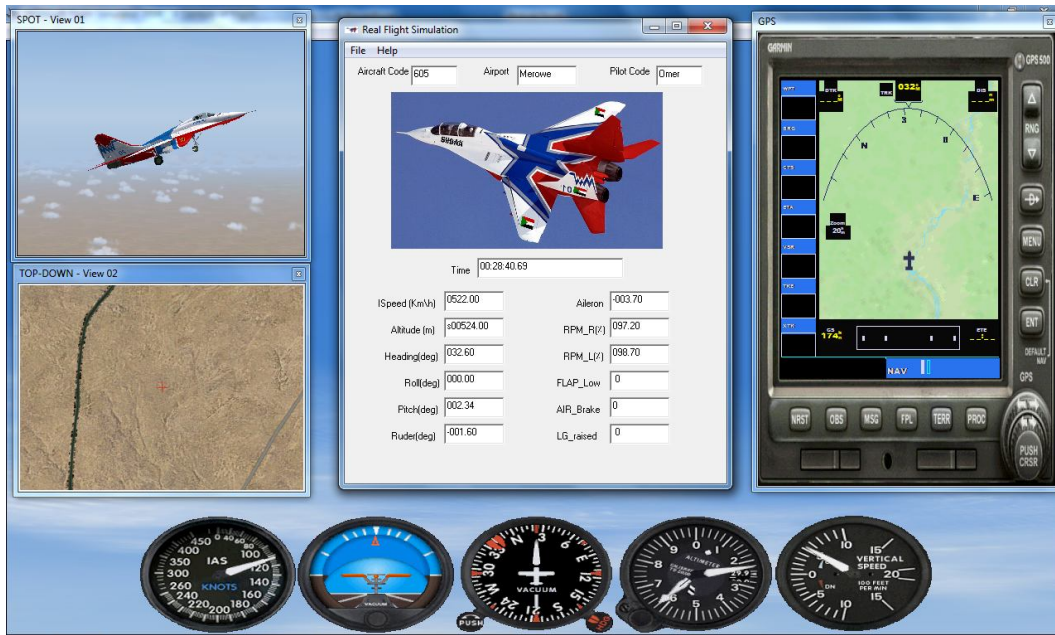
Figure (4.6-c): Combination of the Spot, Top-Down, Real Flight Simulation and GPS with the main window Cockpit View-Basic instruments
