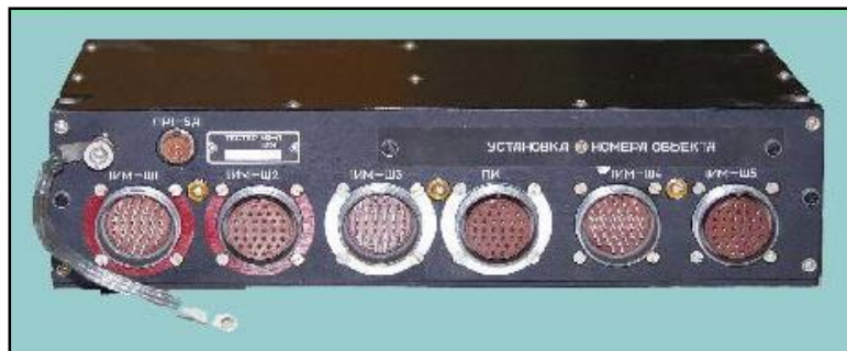
Figure (2.47): Electrical unit (1 IM)
