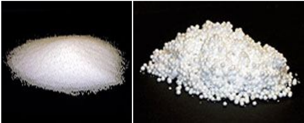
Figure 4-1 Beads of polystyrene before and after pre-expansion process Source: www.Eps-system.com
