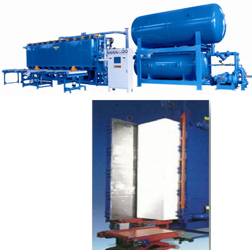
Figure 2-8EPS block mould and vacuum installation.
