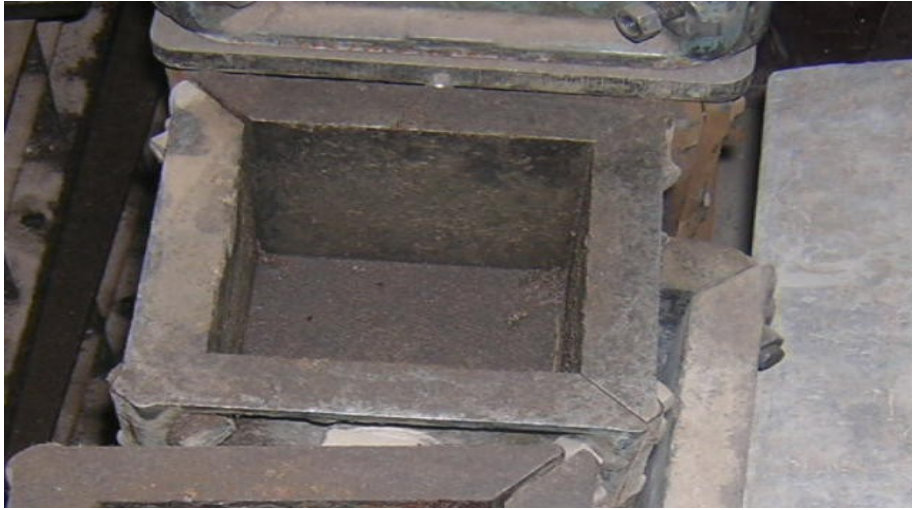
Plate B4: Tight empty 10 cm 3 Mold
