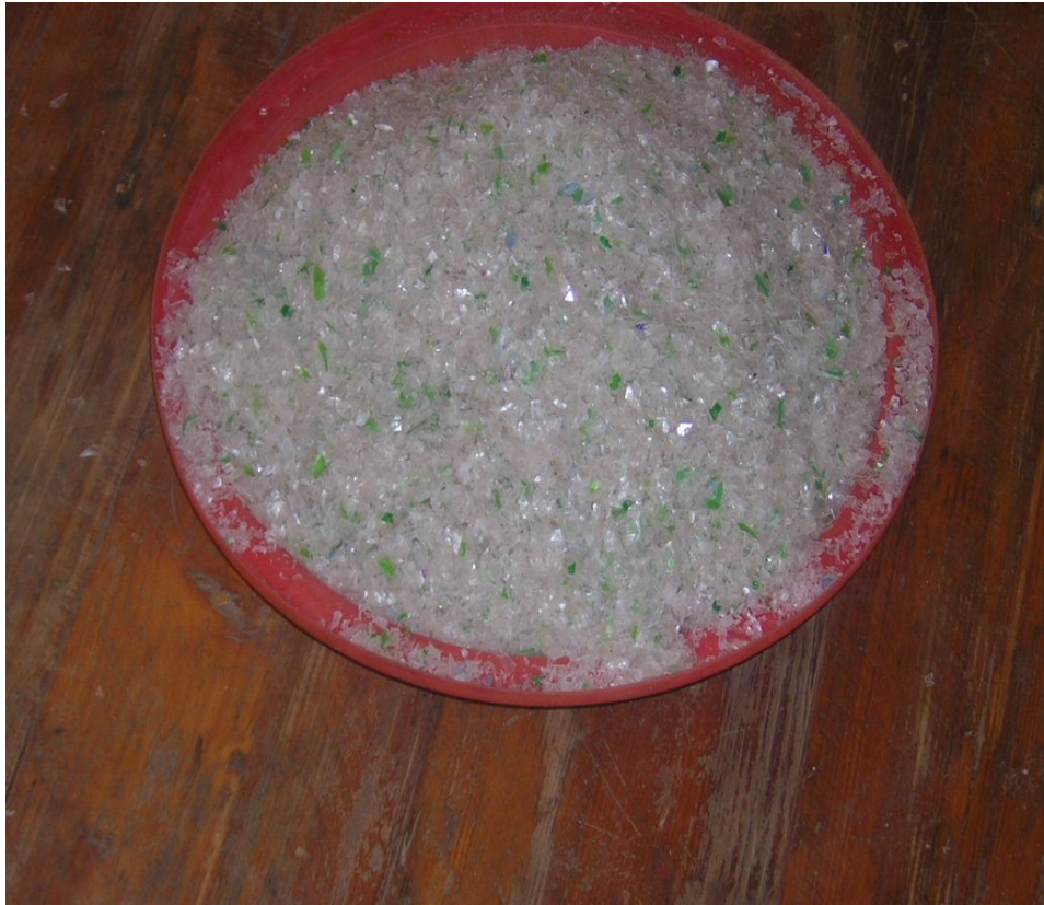
Plate A2: 6.35mm PET material size
