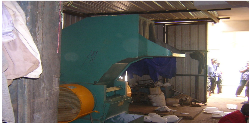
Plate B8: Plastic crushing machine
