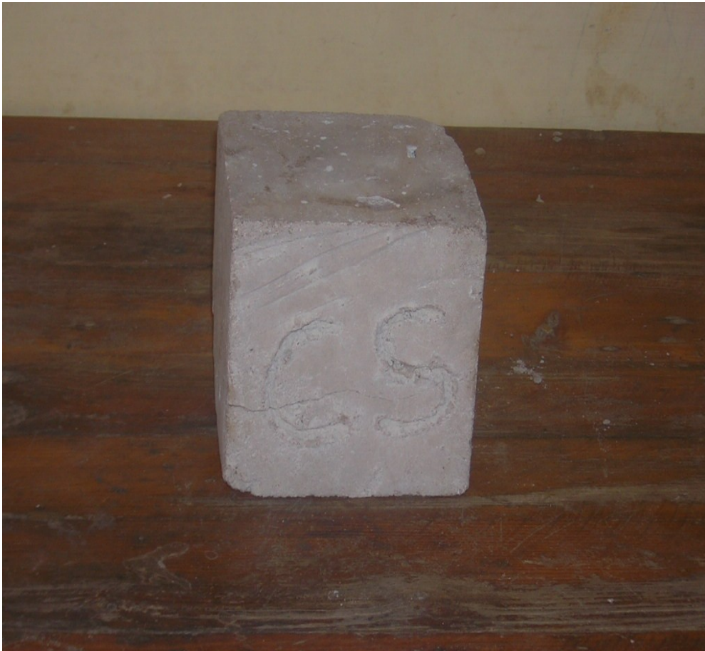
Plate C1: Control Sample Block, S1
