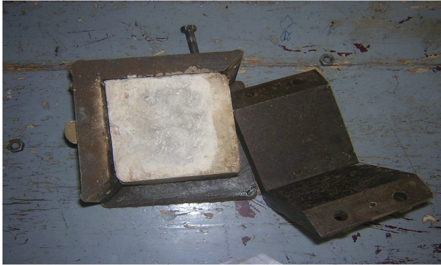
Plate B6: loosed filled 10 cm 3 Mold
