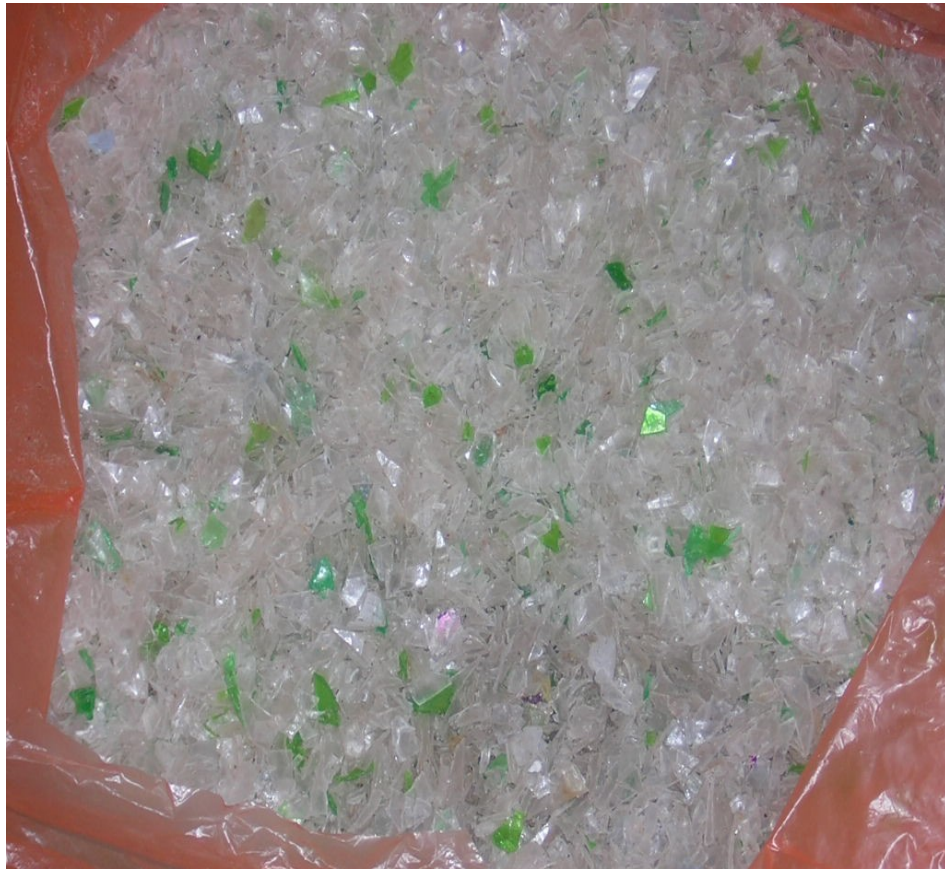
Plate A3: 9.5mm PET material size
