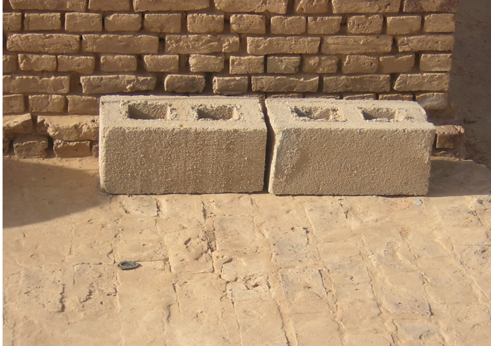
Plate C10: Test sample blocks after curing
