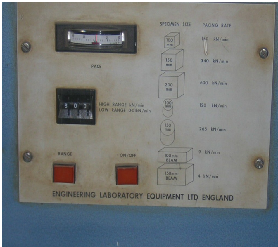
Plate B2: Compressive Strength Tester specifications
