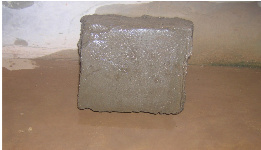
Plate C9: control sample brick after curing
