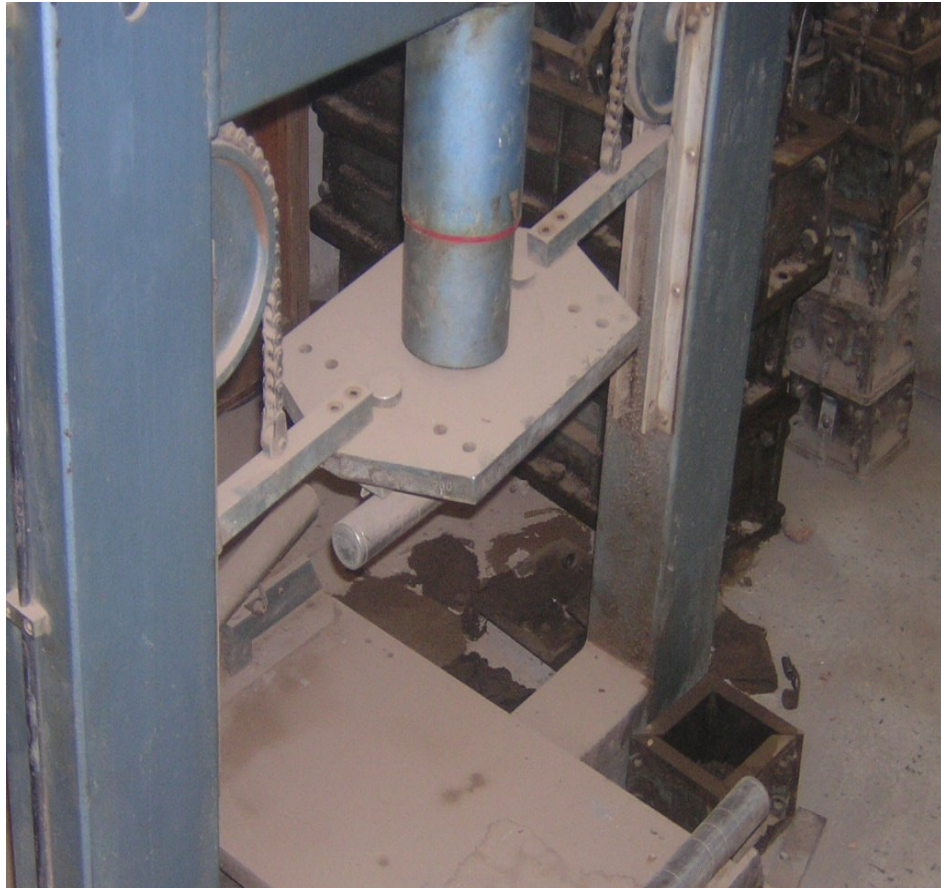
Plate B3: Splitting Strength Tester type: Engineering laboratory equipment LTD
