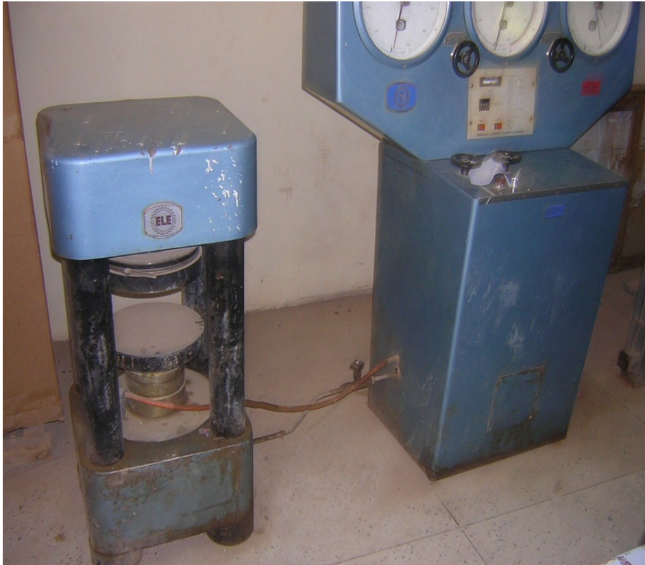
Plate B1: Compressive Strength Tester type: Engineering laboratory equipment LTD
