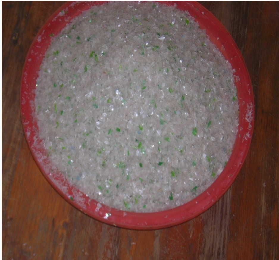
Plate A1: 4.76mm PET material size
