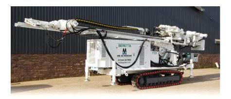
Beretta T151 drill rig, built in Milan by Beretta Alfredo srl, this compact tracked rig powered by a 98kW Deutz engine, it has a small footprint, and can even be operated by remote radio control if needs be.
