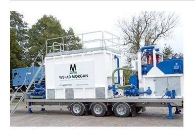
MC80 mobile high performance mud cleaner. Mounted on a 14m trailer, the unit includes a double deck VSM 300, fifth generation, shaker mounted on a hollow section steel frame with underflow tank, mud feed chute, clean mud compartment, Svedala 100 x 75 centrifugal hydrocyclone feed pump with 22 kw motor, 4 No. 5" hydrocyclones, interconnecting pipework, fold-up front access platform, 3 phase compressor, electrical controls and 15m of armoured power cable.
