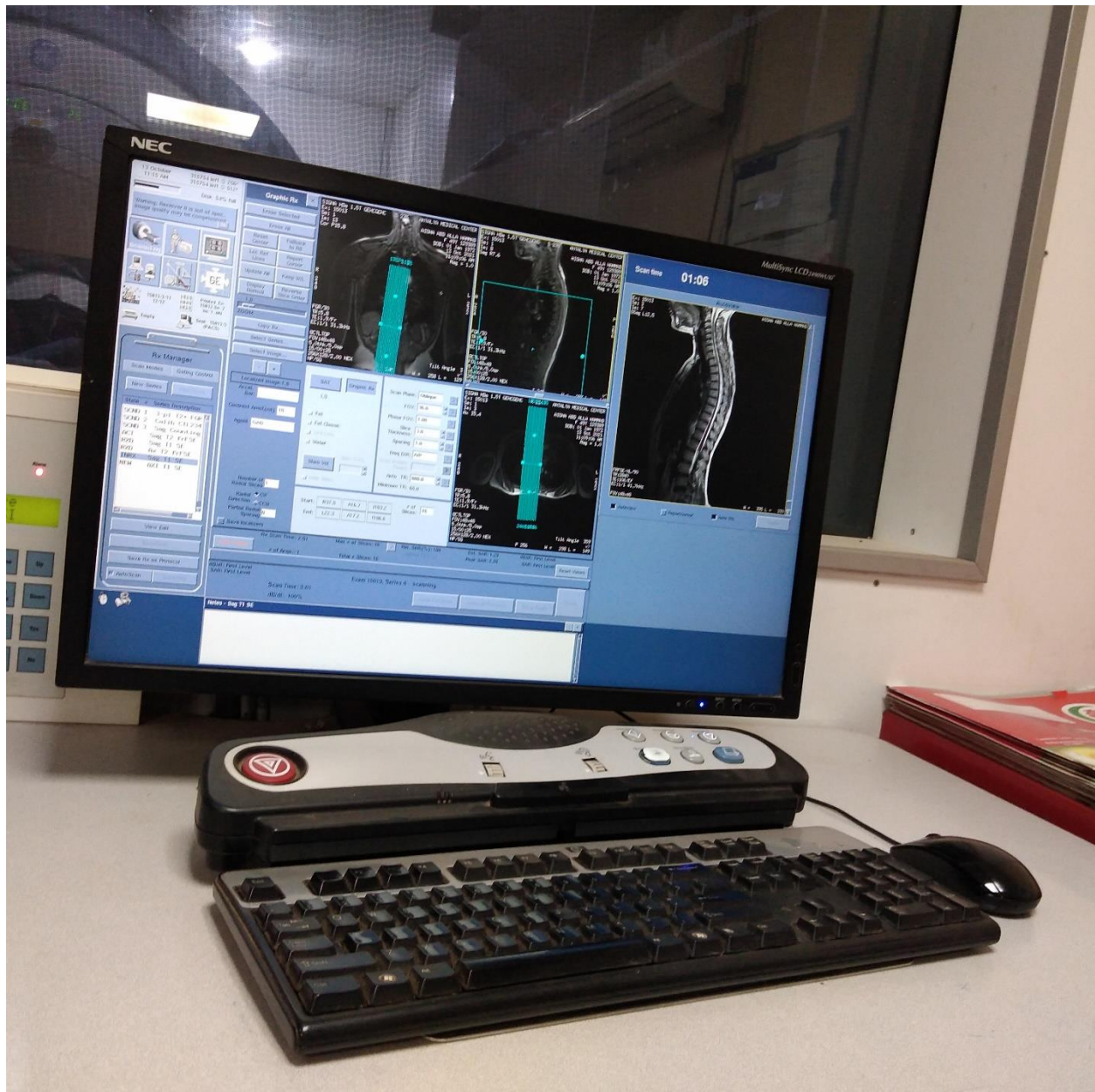
Figure 3.2 shows operating console of MRI machine (GE 1.5 Tesla) in INTALIA MEDICAL CENTER
