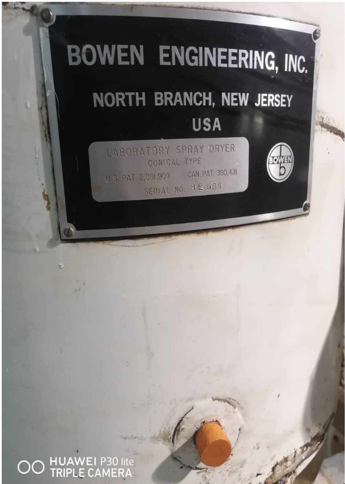
Figure (4.7): The drying machine of NaCl (side view)
