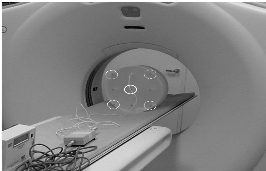
Fig ( 2.7 ) : Dose measurement setup with CTDI body phantom (32-cm diameter) and ion chamber (100-mm length) (Jiang 2009).
