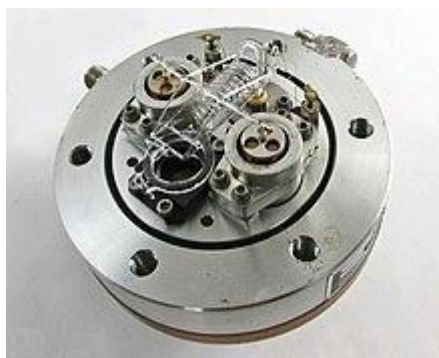
Figure (3.2): A Force-Balanced Fused Quartz Bourdon Tube Pressure Sensor , the mirror that should be mounted to the armature is absent.
