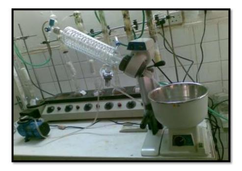
Plate No.7 Soxhlet and Rotary evaporator
