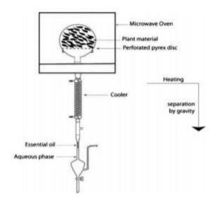
Fig.1.7: Apparatus for microwave hydro diffusion and gravity
