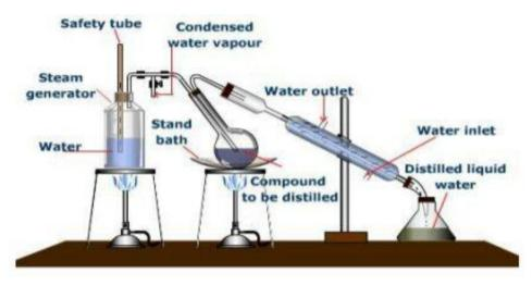
Fig.1.2 : Schematic of apparatus for Steam distillation
