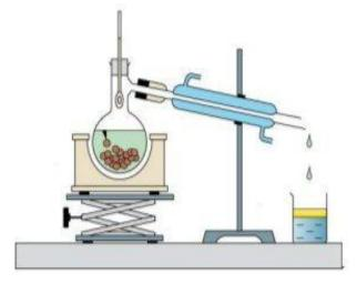
Fig.1.1: Schematic of apparatus for hydrodistillation
