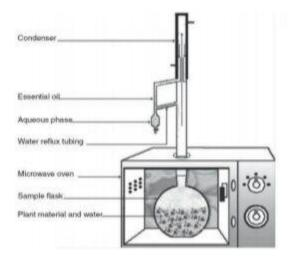
Fig.1.5: Apparatus of microwave-assisted hydrodistillation
