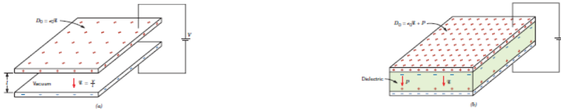
Figure (2.5) A parallel-plate capacitor (a) when a vacuum is present and (b) when a dielectric material is present.
