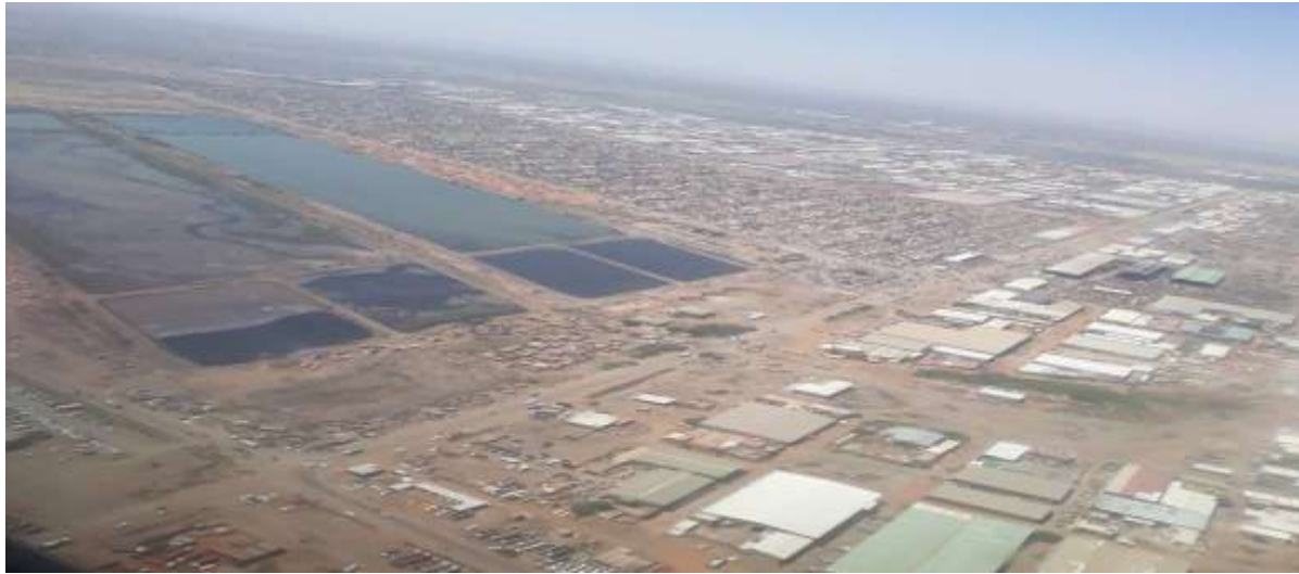
Figure (1 .3) Showing the treatment of sewage water inside Soba treatment plant (outlet) by the stabilization bond
