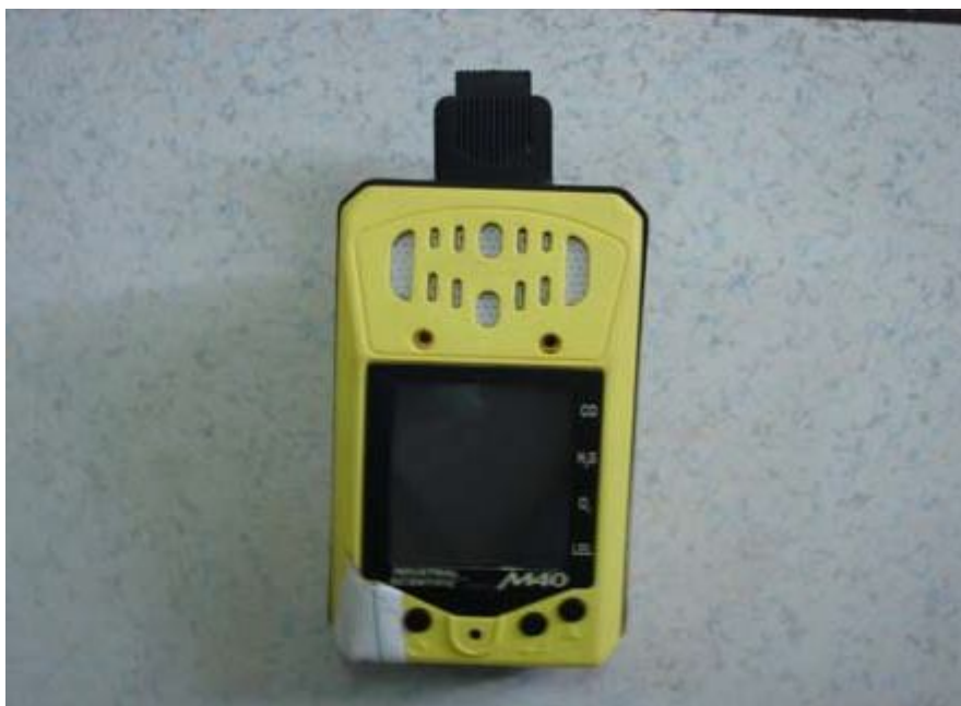
Figure 3-4: M40 used for reading CO in KRC
