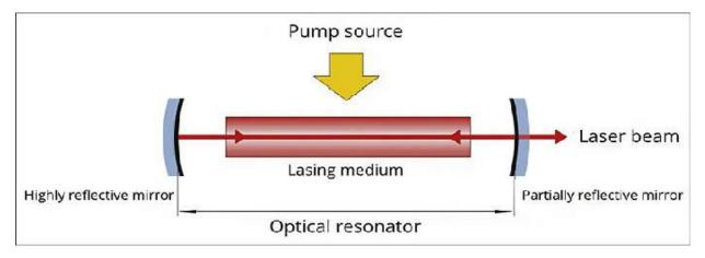
Figure 2: Schematic drawing showing the main components of a laser
