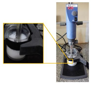
Figure 3-6: Sonication of silica nanoparticles in PVA solution.
