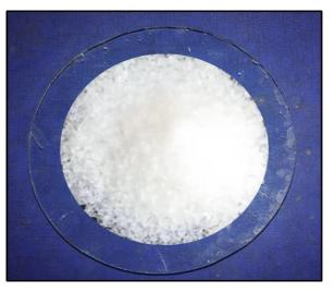
Figure 3-2. Polyvinyl alcohol (PVA) powder.
