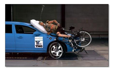
Figure 2-5. Pedestrian protection airbag (Maki et al., 2003).
