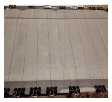
Figure 3-7: Dip-coated nylon 66 by PVA/silica nanoparticles.
