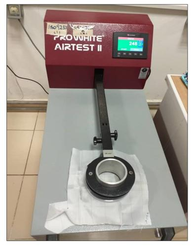
Figure 4-6: Air permeability tester.
