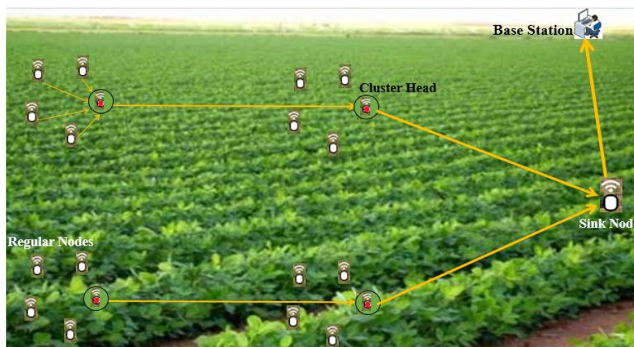
Figure 2.5. Precision agriculture architecture for monitoring applications using the multi-hop clustering model in WSNs.
