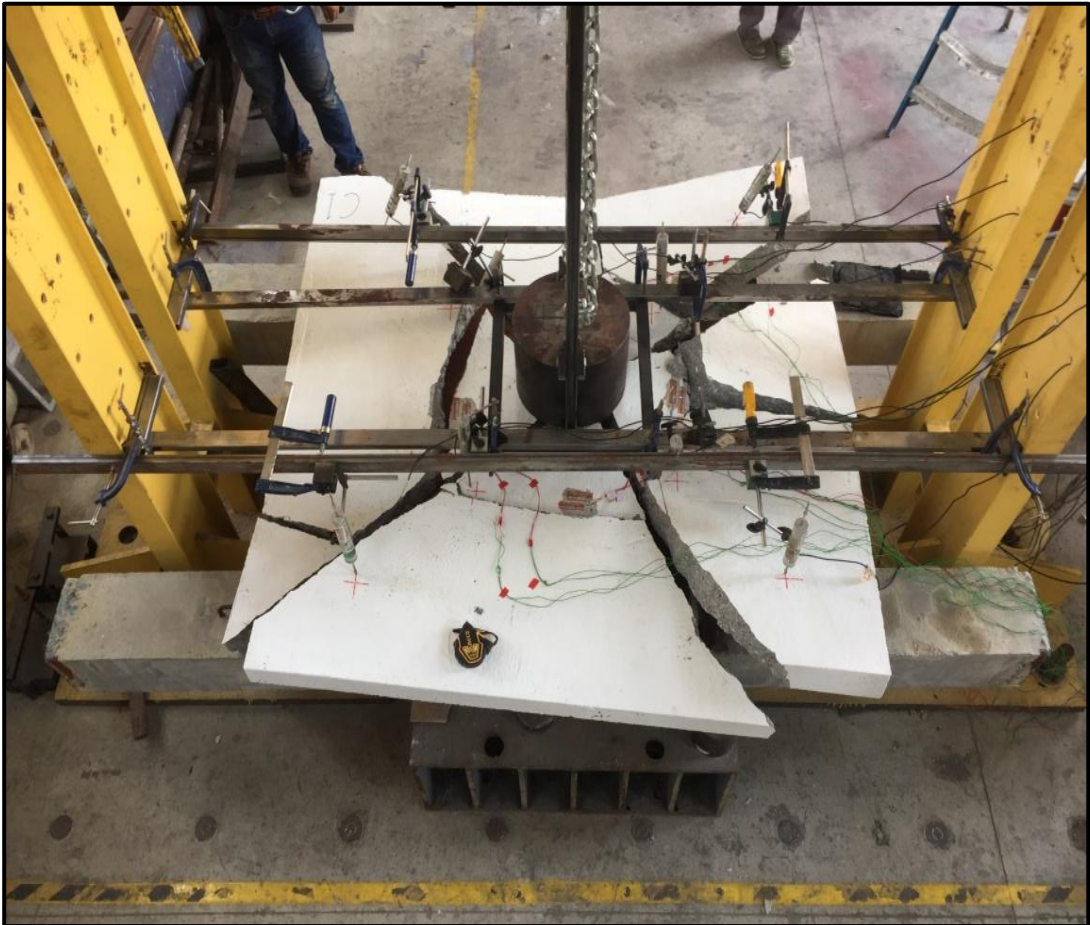
Figure 4.62 Final Crack Patterns for Impact Test Specimen C1
