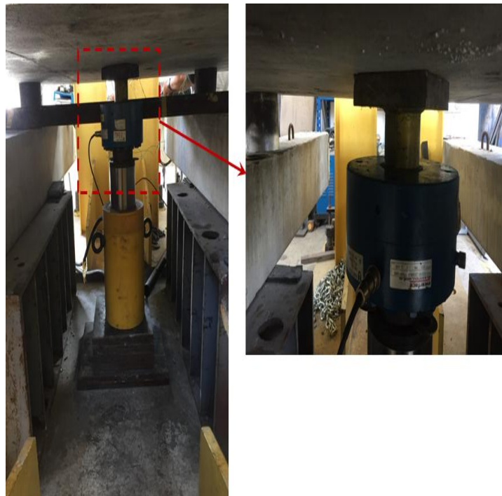
Figure 3.16 Load Cell Placed at the Center Soffit Slab
