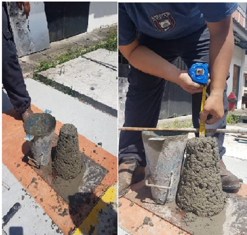
Figure 3.3 Concrete Slump Tests
