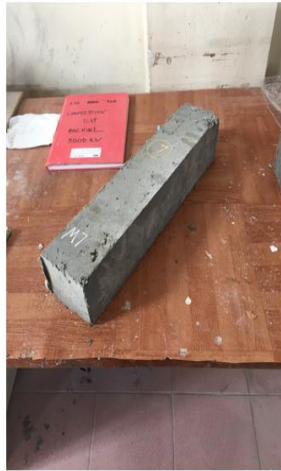
Prism condition (before tested)
