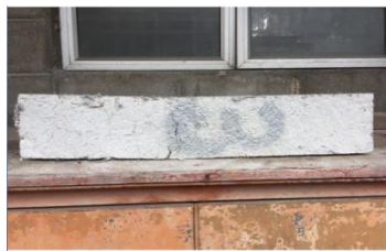
Prism failure (right view) – only cracks appeared
