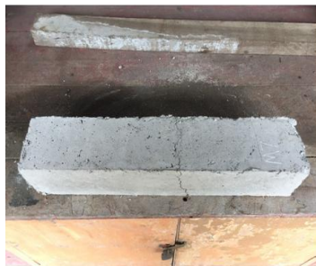
Prism failure (plan view) – only cracks appeared
