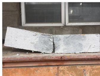
Prism failure (right view) – almost splitted into two sections
