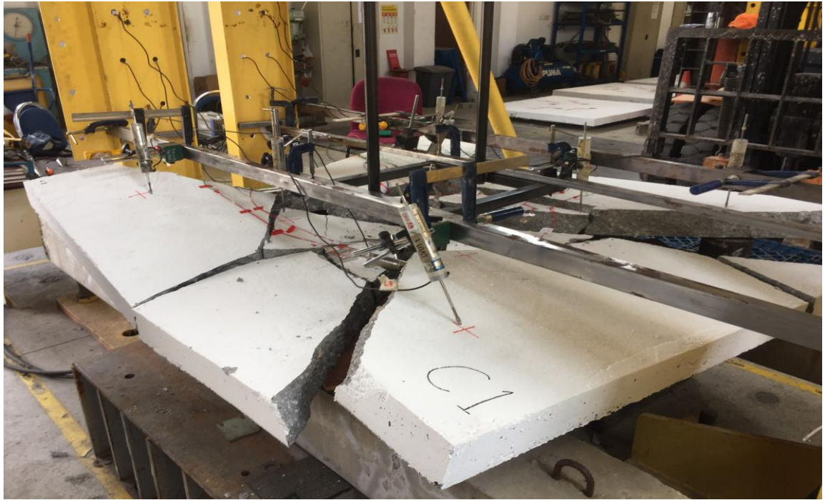
Figure B1: Failure for Slab Specimen C1 (1m drop) – side view
