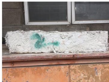
Prism failure (right view) – only cracks appeared
