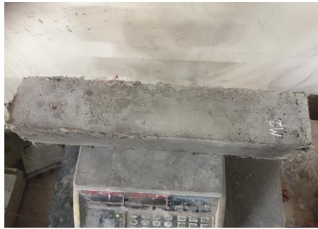
Prism condition (before tested)
