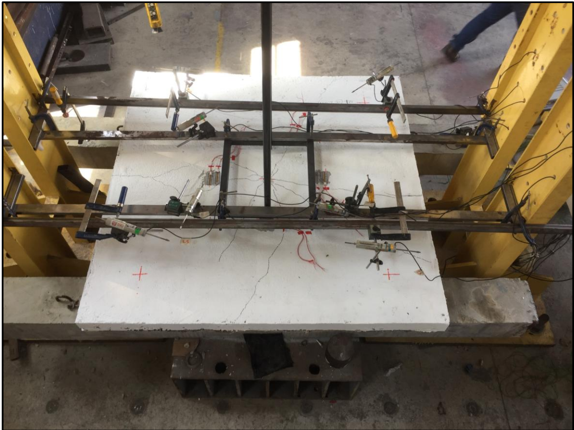
Figure 4.63 Final Crack Patterns for Impact Test Specimen M1
