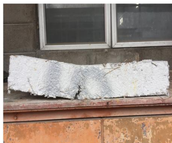
Prism failure (right view) – almost splitted into two sections
