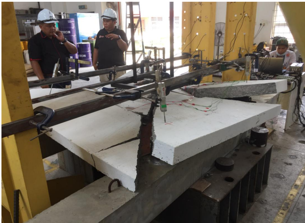
Figure B2: Failure for Slab Specimen C1 (1m drop) – other side view
