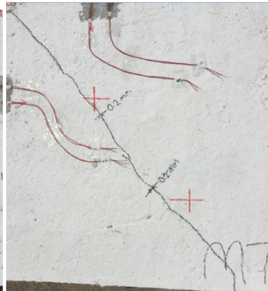
Figure B9: Failure for Slab Specimen M7 (2m drop) – another plan view (0.1, 0.2, 1.4 and 1.6 mm crack widths)
