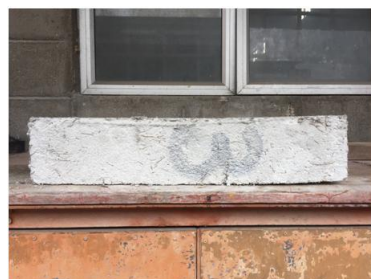
Prism failure (right view) – only cracks appeared
