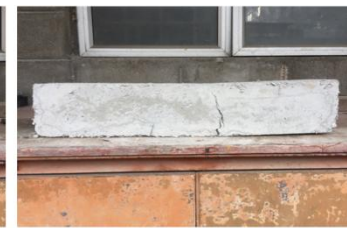
Prism failure (left view) – only cracks appeared
