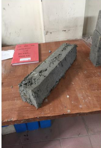
Prism condition (before tested)
