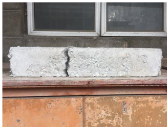
Prism failure (right view) – splitted into two sections
