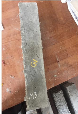
Prism condition (before tested)
