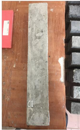
Prism condition (before tested)
