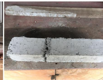
Prism failure (left view) – splitted into two sections
