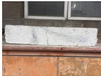
Prism failure (right view) – only cracks appeared
