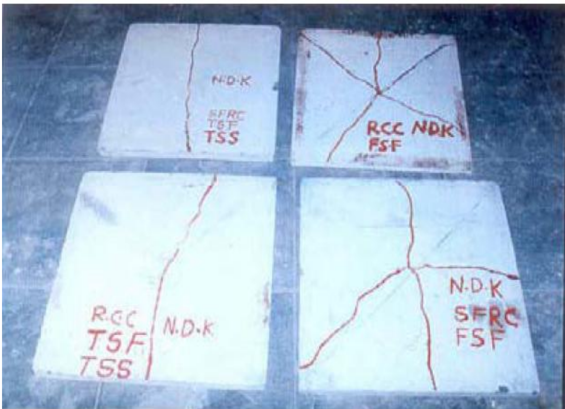
Figure 2.30 Cracking Patterns of Plates (Elavenil & Knight, 2012)
