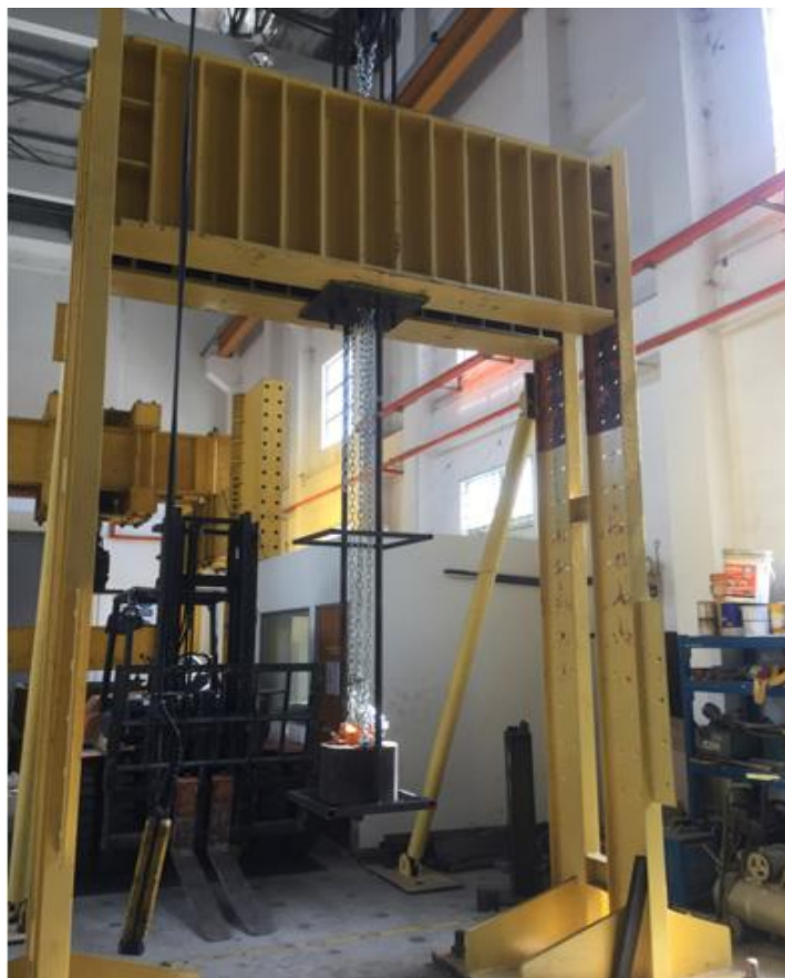
Figure A5: Setting up glider and mass of 200 kg into the frame
