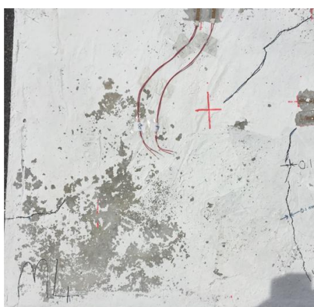
Figure B6: Failure for Slab Specimen M4 (2m drop) – another plan view (0.1mm crack width)
