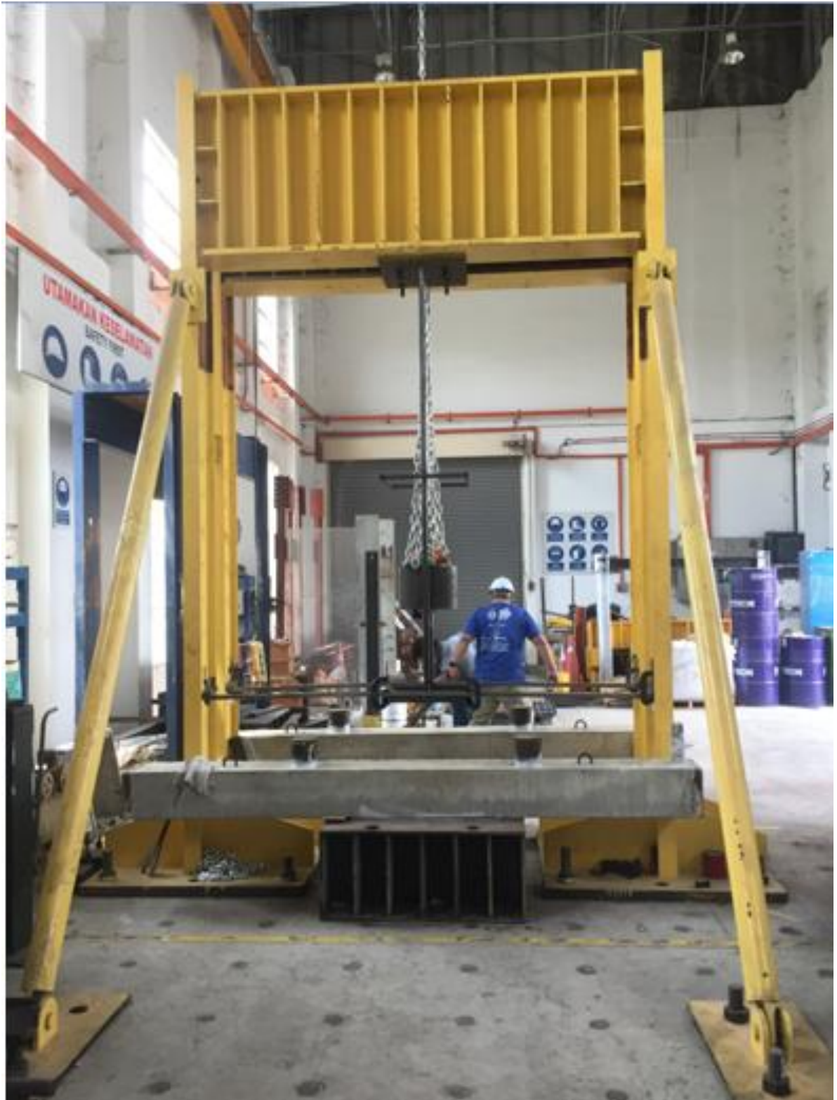
Figure A6: Complete Frame Set Up for Impact Load Test
