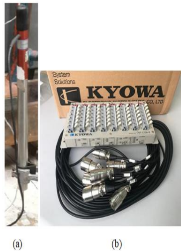
Figure 3.17 the Instruments Used in the Impact Test; (a) the LVDT and (b) the Data Logger System
