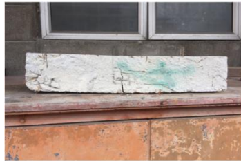
Prism failure (right view) – only cracks appeared
