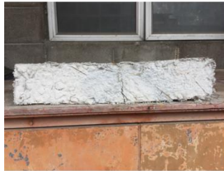
Prism failure (right view) – only cracks appeared
