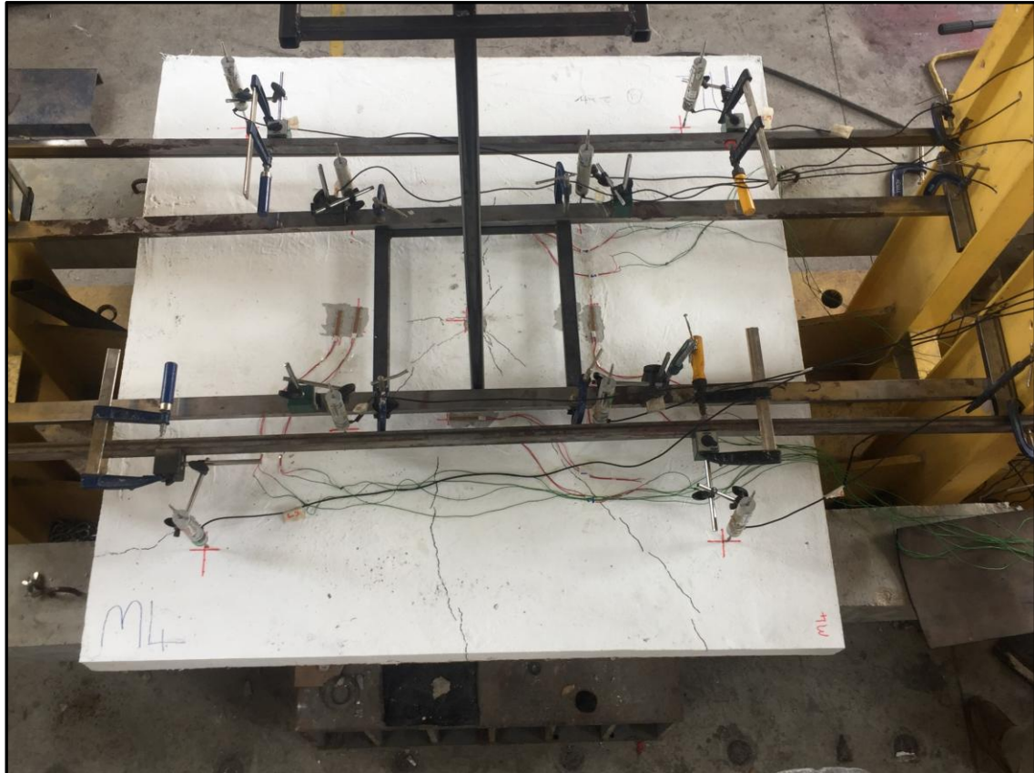
Figure 4.66 Final Crack Patterns for Impact Test Specimen M4
