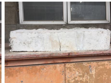
Prism failure (left view) – only cracks appeared
