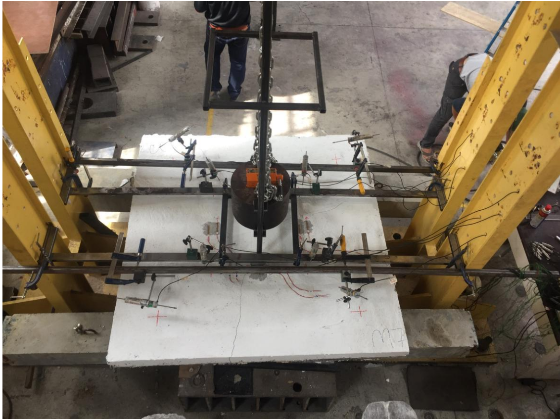
Figure 4.69 Final Crack Patterns for Impact Test Specimen M7
