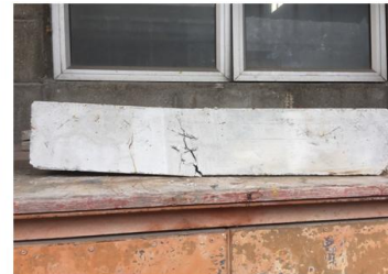
Prism failure (left view) – only cracks appeared
