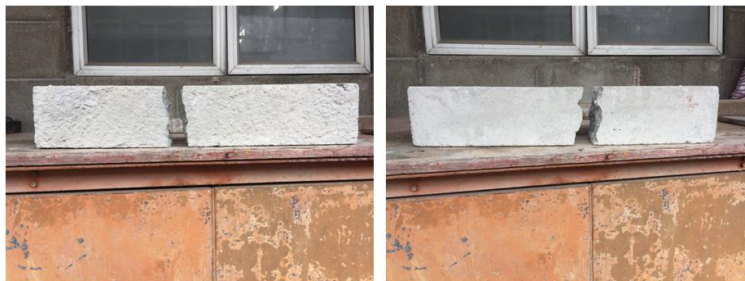
Prism failure (right view) – splitted into two sections
