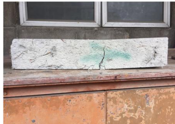
Prism failure (right view) – only cracks appeared
