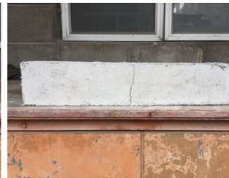
Prism failure (left view) – only cracks appeared
