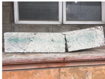
Prism failure (right view) – almost splitted into two sections
