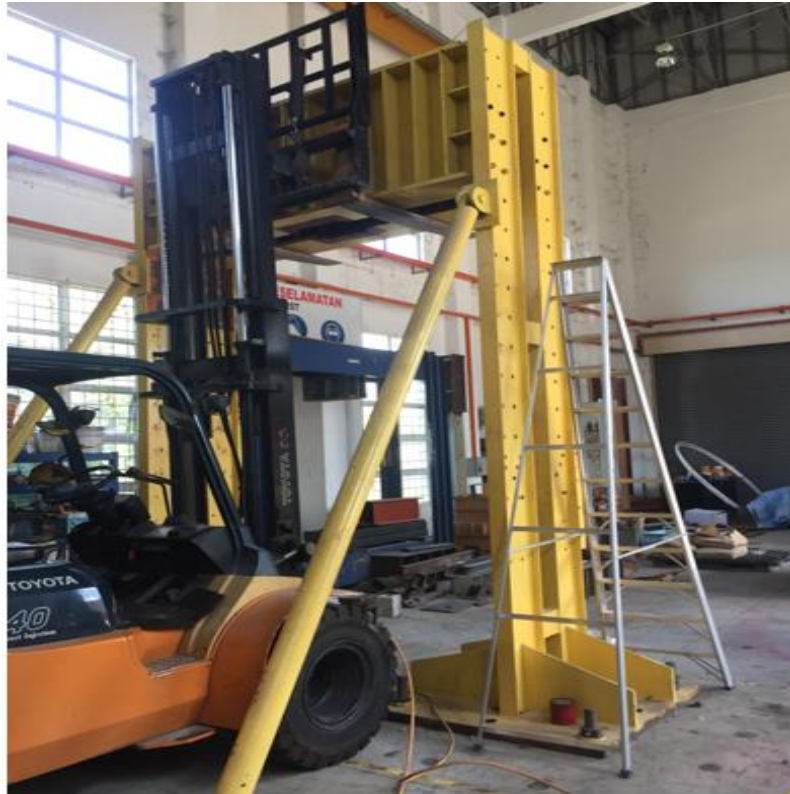
Figure A2: Adjustment the Frame of Impact Load Test with Height with Max. 2 m Free Fall
