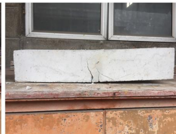
Prism failure (left view) – only cracks appeared
