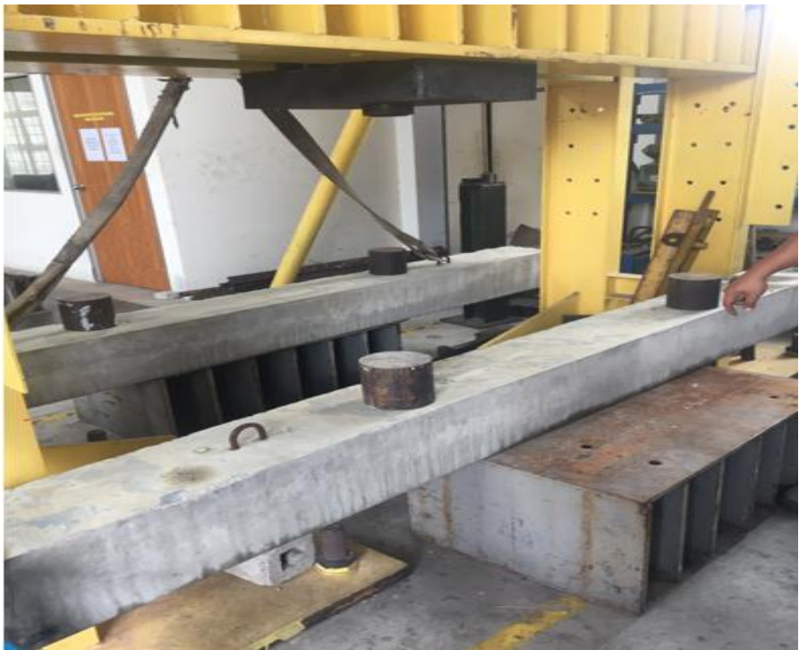
Figure A1: Setting for Slab's Support
