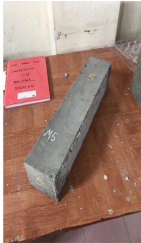
Prism condition (before tested)
