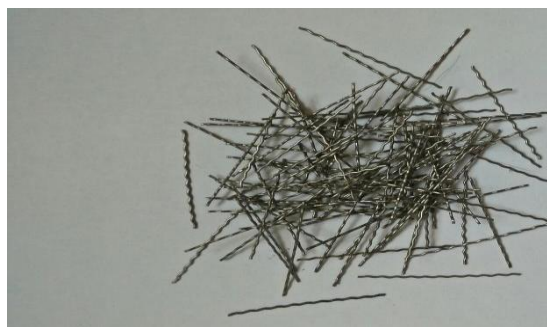
Figure 2.17 Steel Fiber (Prakash, 2017)
