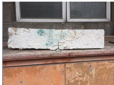
Prism failure (right view) – only cracks appeared
