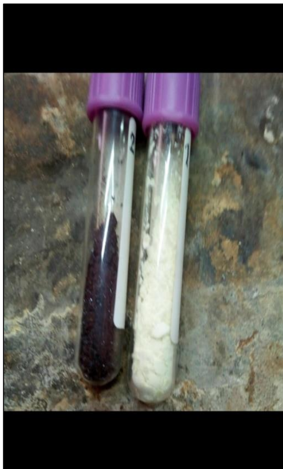
Figure (4.4): Nano powder form for two samples of (\text{Ba}_x\text{Fe}_{1-x}\text{TiO}_4) ( x= 1, 0.1, 0.2, 0.3, 0.5, 0.6, 0.7, 0.8, 0.9 and 0 ) samples.
