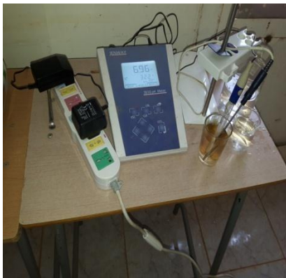
Figure(4.3.2) :Conductivity meter and measurement of conductivity
