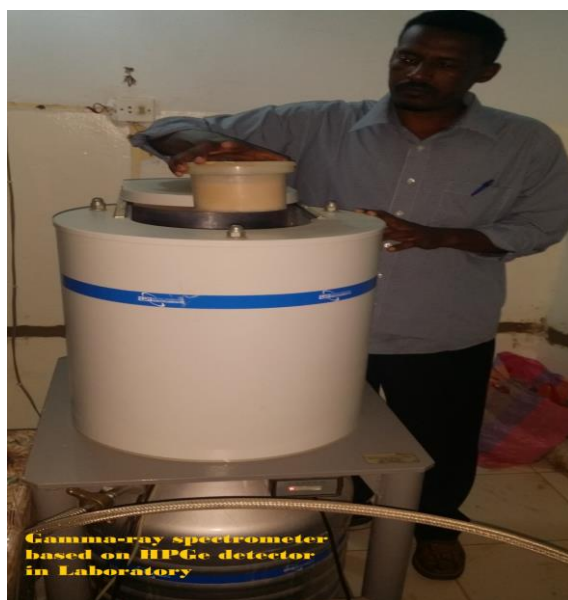
Figure 3.4: Analysis of Samples in the Laboratory Sudanese Atomic Energy Agency in Khartoum by Gamma-Ray Spectrometer.
