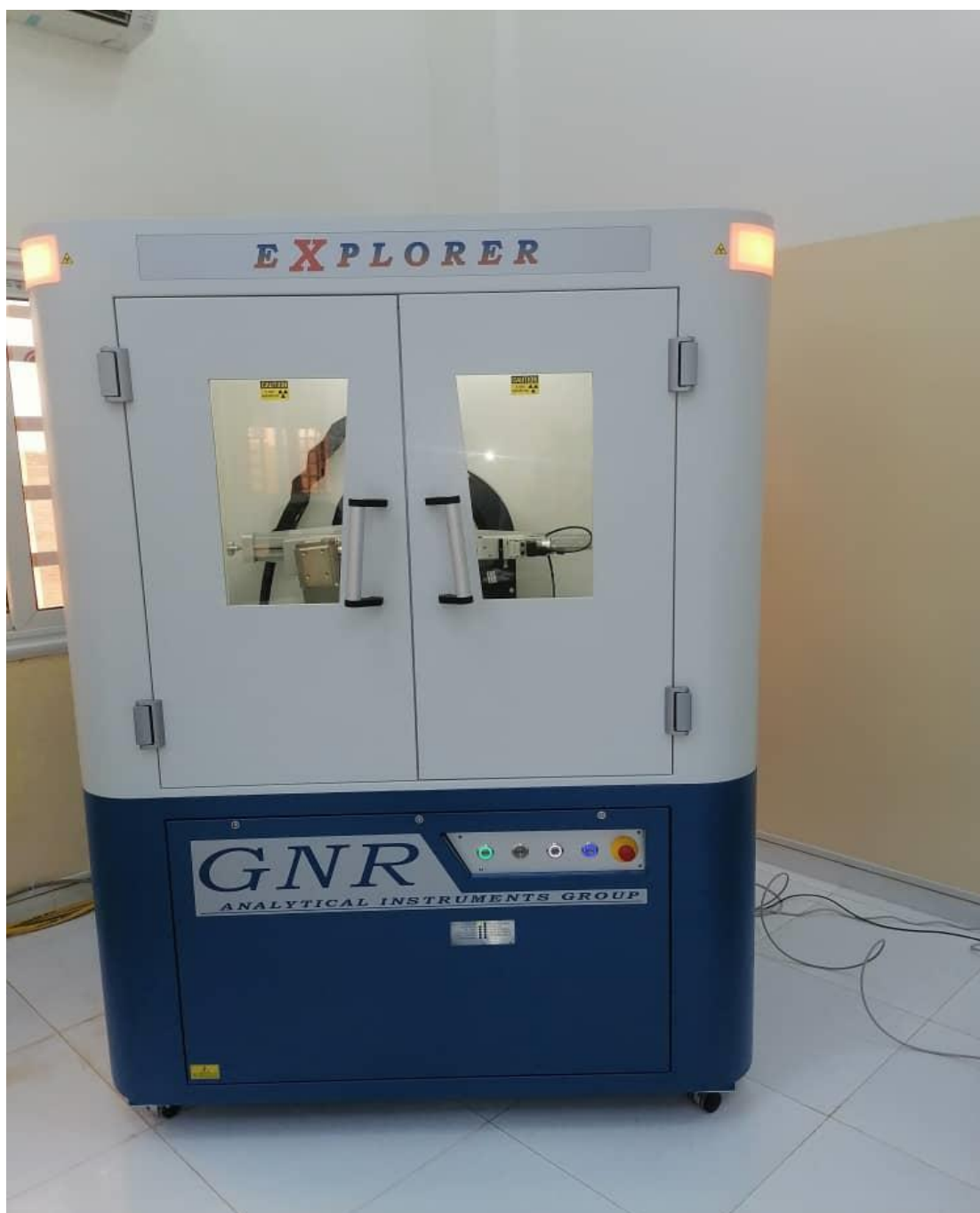
Figure (3.15): The XRD apparatus used for structural analysis in this study.
