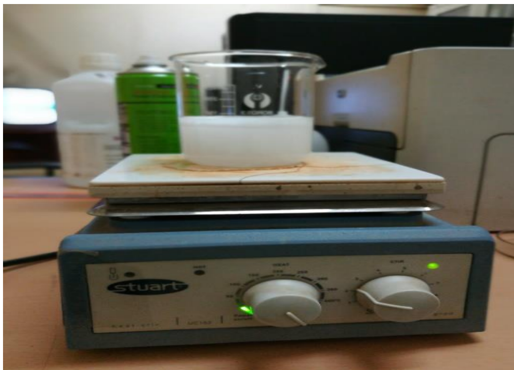
Figure (3.7): The magnetic stirrer instrument used in this study.
