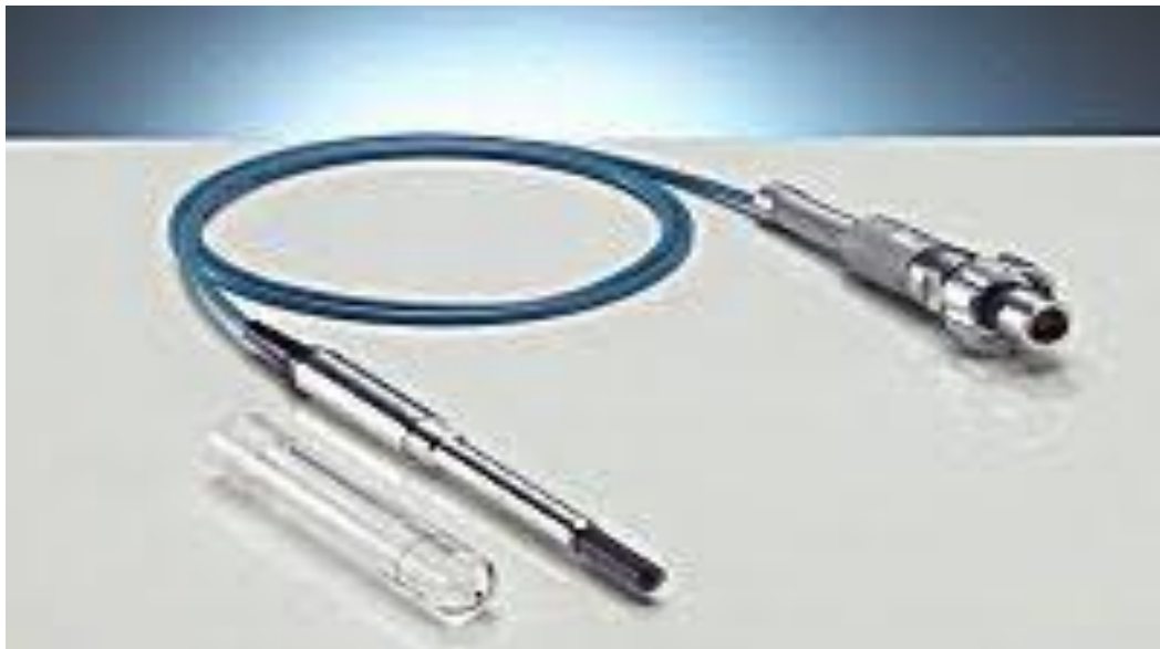
Figure (3.11): The ionization chamber used in this study.
