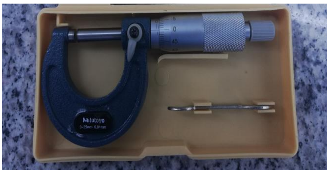
Figure (3.8): The micrometer Instrument used in this study.
