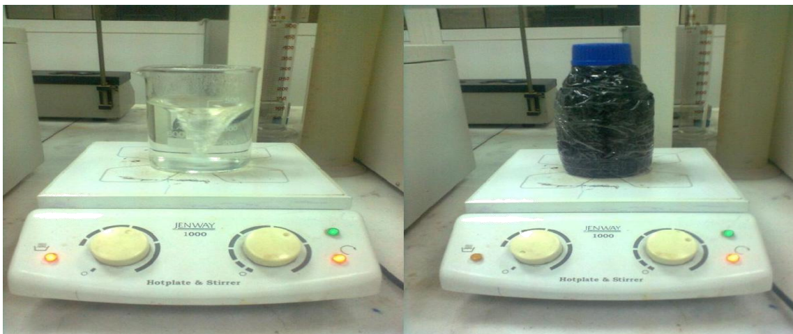
Figure (3.17): The dissolution of PVA/AgNO 3 in distilled water using magnetic stirrer and a hotplate.
