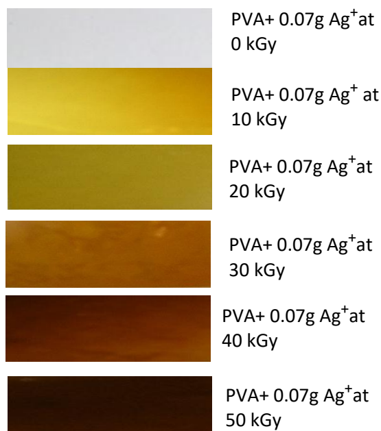
Figure (2.23): The color change to golden yellow of irradiated PVA/AgNO 3 composites due to reduction of AgNO 3 to Ag + nanoparticles induced by \gamma -rays. The picture of the un-irradiated film was taken on a white background.
