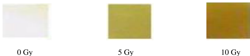
Figure (4.1): The change in PVA/AgNO 3 films color intensity due to irradiation with \gamma -ray doses.
