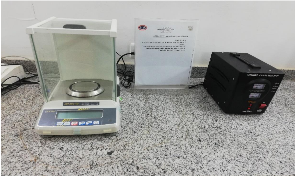
Figure (3.5): The sensitive balance used in this study.
