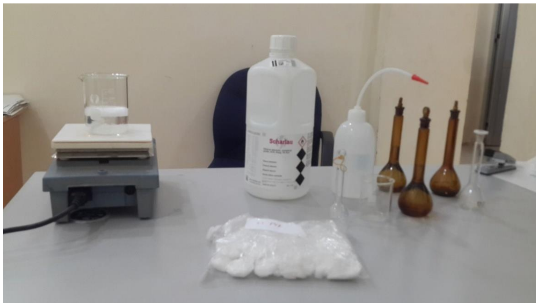
Figure (3.16): Some tools used during PVA/AgNO 3 synthesis.
