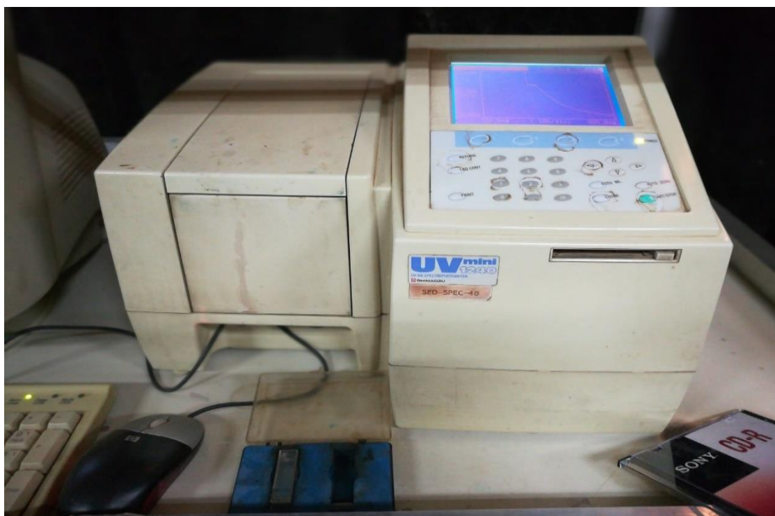
Figure (3.4): The UV- Visible spectrophotometer used in this study.
