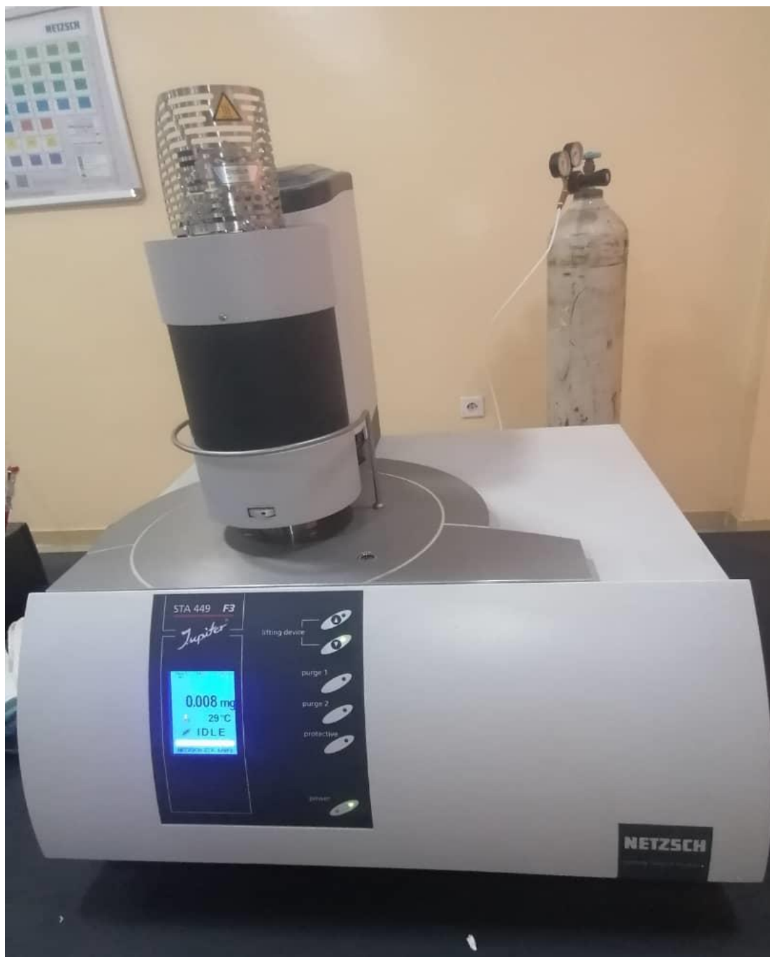
Figure (3.14): The apparatus used for thermal analysis in this study.
