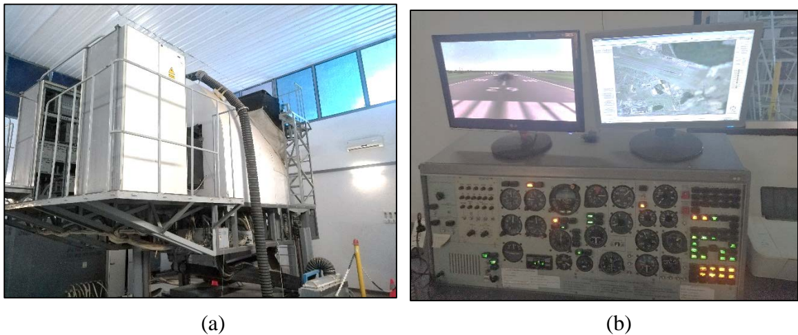
Figure 3-16: (a) Antonov AN-26B Simulator Using (b) Xplane Visual Engine
