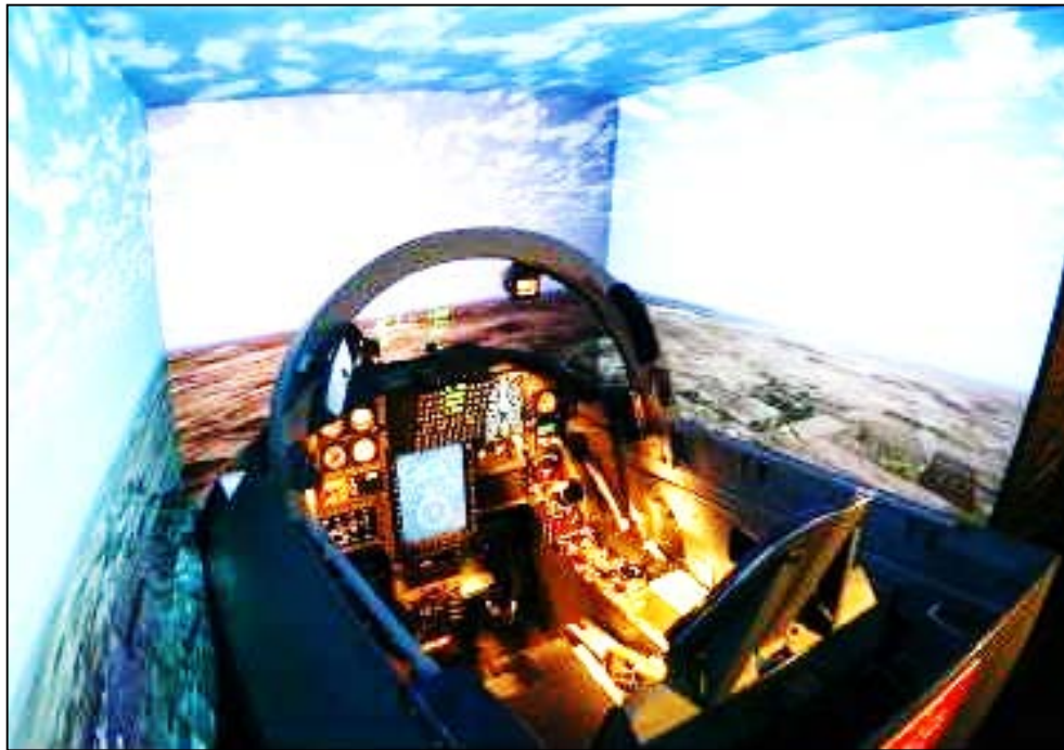
Figure 3-24: A Flight Simulator Used by USAF Utilizing CAVE Concept [1]
