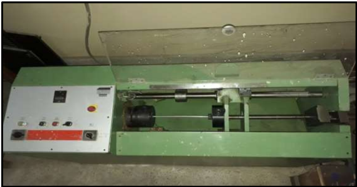
Figure (3-7): Machine of buckling test-rig used in this work
