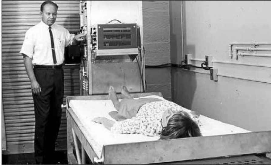
Figure 2.2: Hal Anger in 1965 with the whole-body scintillation scanner at the Donner Laboratory. The small holes in the foreground are part of the collimator. From the collection of Henry N. Wagner, Jr., MD.
