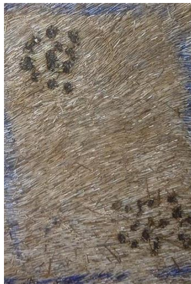
Figure 4.1: Nd: YAG laser effect on leather.
