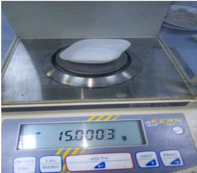
Figure 4.4: Preparation of coating material: a) NaCl powder b) prepared suspension
