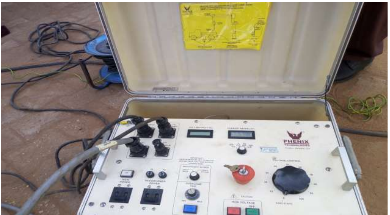
Figure 4.10: single phase 100KV Transformer control test unit
