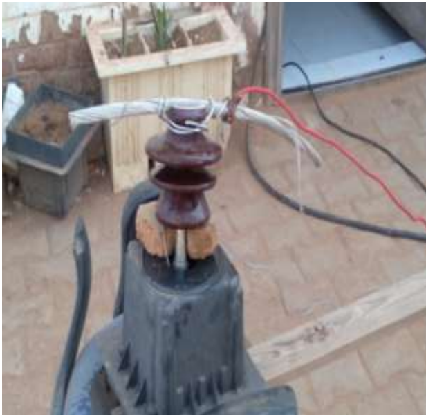
Figure 4.11: test object connection: a) ceramic b) polymer
