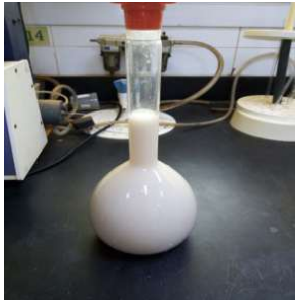
Figure 4.4: Preparation of coating material: a) NaCl powder b) prepared suspension
