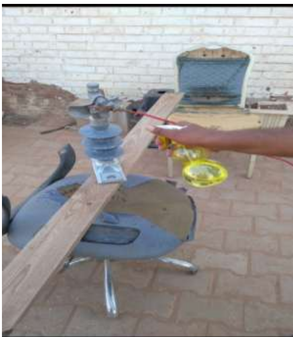
Figure 4.12: test object wetting procedure
