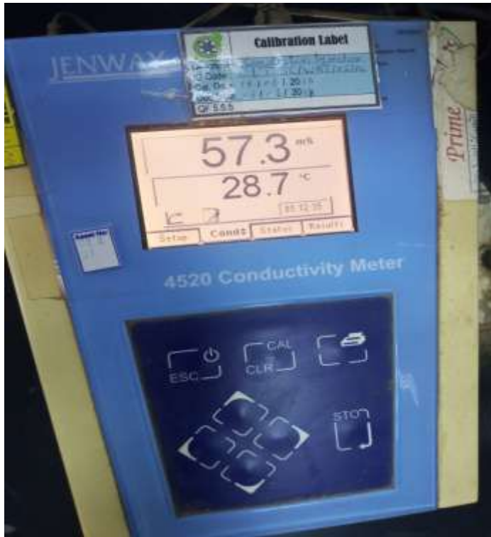
Figure 4.9: wet test solution: a) conductivity reading b) prepared solution
