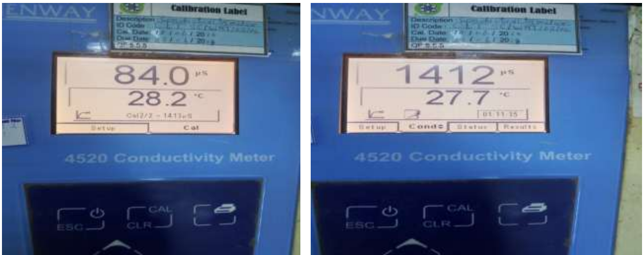
Figure 4.5: Calibration of conductivity meter probe: a) 84 \mu\text{S} CRM b) 1412 \mu\text{S} CRM
