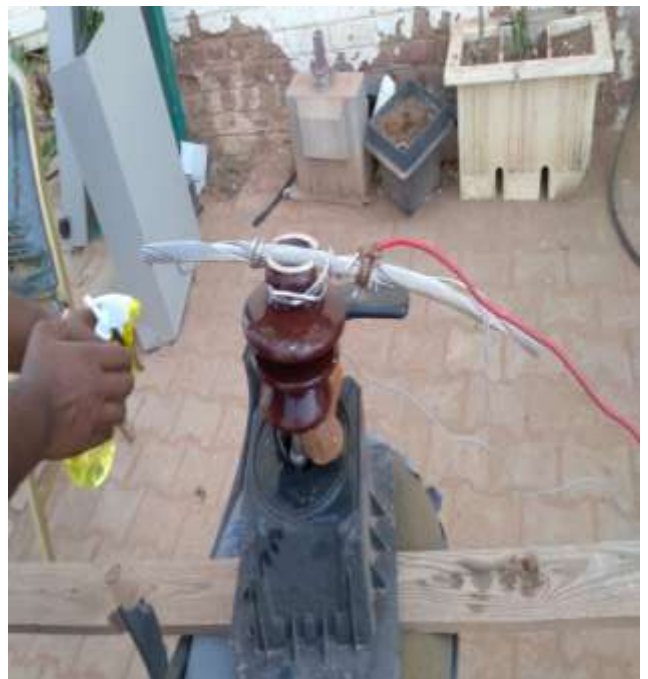
Figure 4.12: test object wetting procedure
