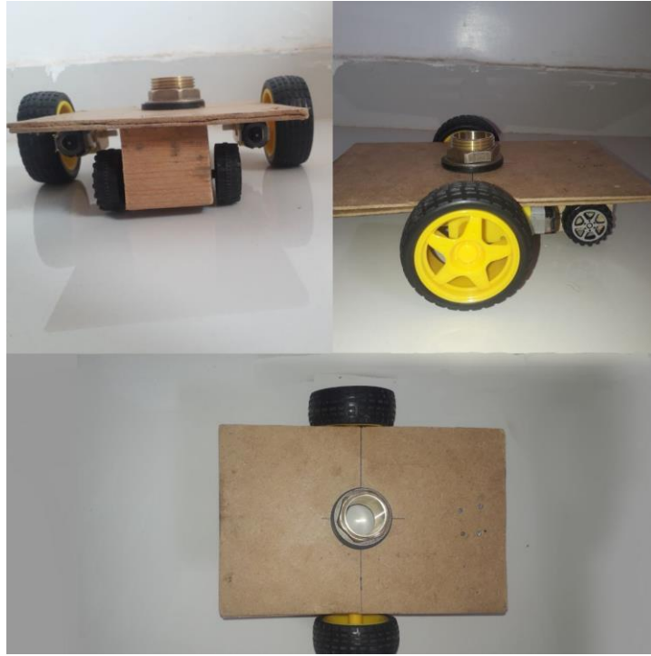
Figure 4.5: Plan, front, and side elevation of chassis
