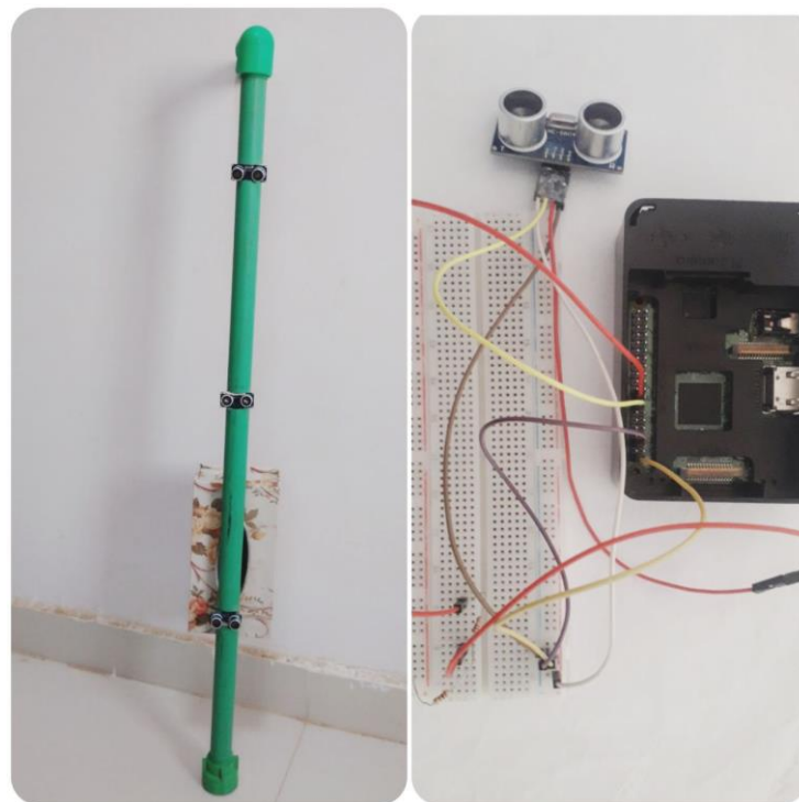
Figure 4.7: Real connection of ultrasonic sensor
