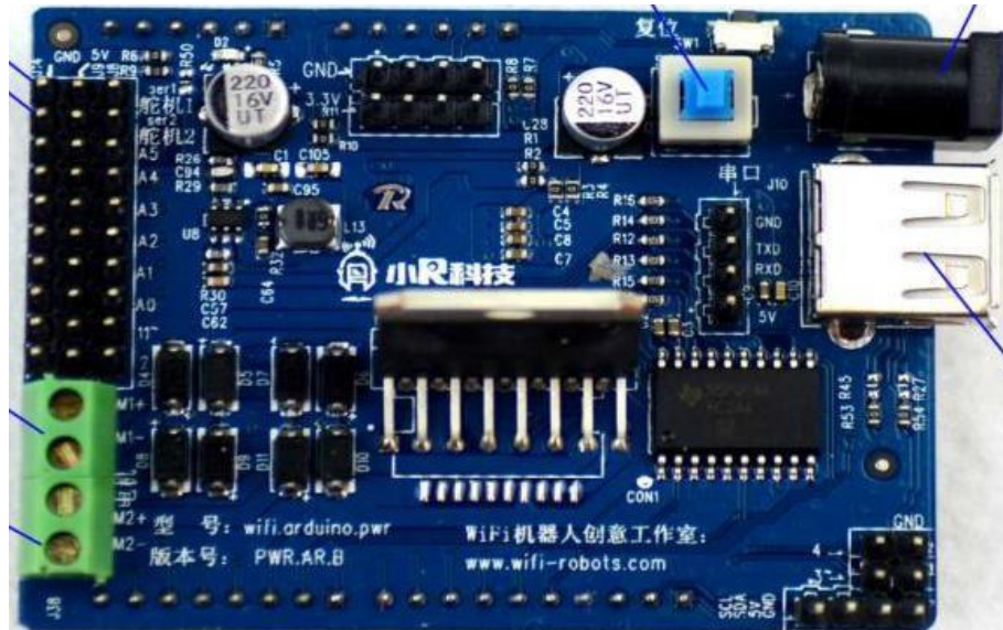
Figure 4.4: L298N Motor shield drive
