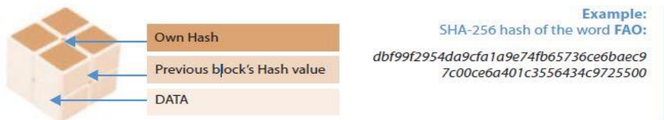
Fig 2. 4. One block (nodes) on the block chain [12]
