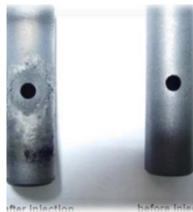
Fig 2.15: photos of a graphite tube before and after injection
