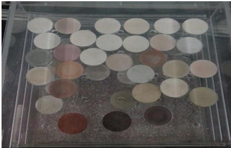
Fig 2.13 : Pressed pellets of samples perior to their analysis by (WDXRF) (c) Sample preparation for SEM + EDXRF technique (non- destructive method )
