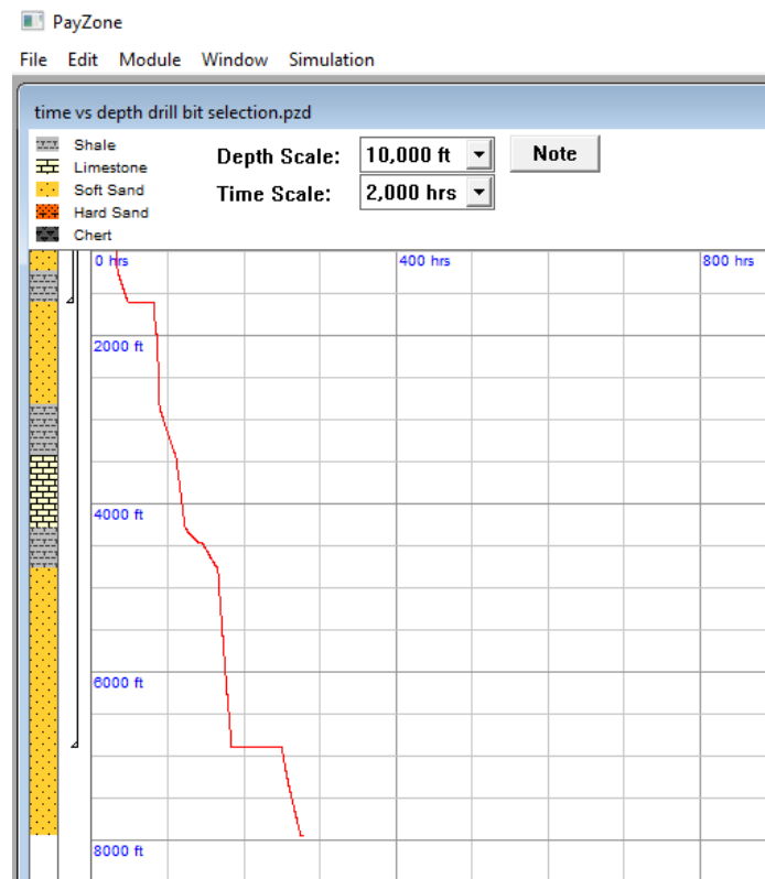
Fig 4.11: Time Vs depth for Bit selection optimization
