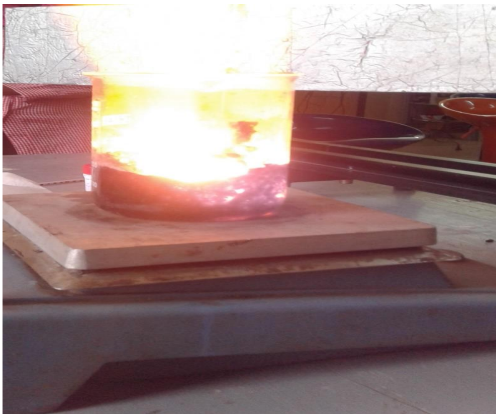
Figure 3.1. Experimental set up of the combustion method for sample 1 at 350 °C, Institute of Laser, Sudan University of Science and Technology, Sudan.
