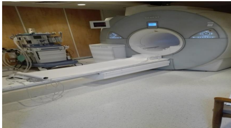
Fig 3.1.1.1 Show Magnetic Resonance device Siemens avanto 1.5 Tesla New when installed in 2013 SaudiGermem hospital
