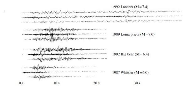
Figure (3.1) Typical earthquake accelerograms
