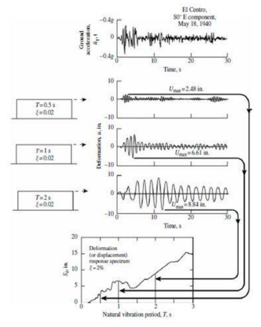
Fig.3.2Computation of deformation (or displacement) response spectrum (Chopra, 1981)
