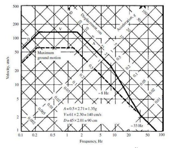
Fig. 3.5 Idealized elastic design spectrum, horizontal motion (ZPA<sup>1</sup>/<sub>4</sub>0.5g, 5% damping, one sigma cumulative probability (Chen and Lui, 2006)
