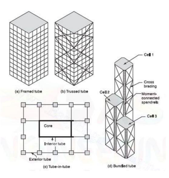
Fig. 2.7 Types of tubes structures (Earthquake Behavior of Buildings, 2012)
