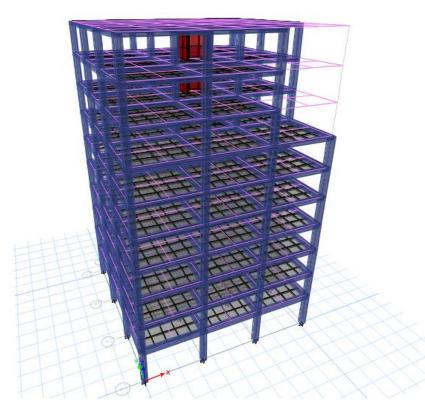
Figure (4.2) 3-D View for 10 Stories RCC Framed Structure
