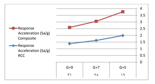
Figure 4.5: Graph of Average Response Acceleration against Number of stories for both models
