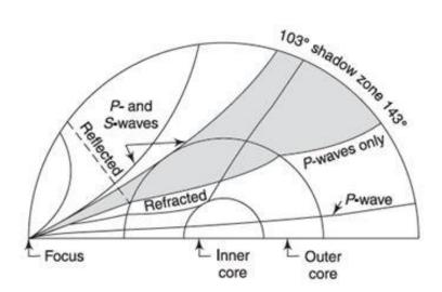
Fig. 2.5 Seismic wave paths (Chen and Lui, 2006)
