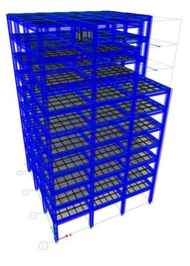
Figure (4.3) 3-D View for 10 Stories Composite Steel Frame Structure
