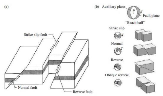
Fig. 2.2 (a) Type of faulting and, (b) focal mechanisms (Chen and Lui, 2006)
