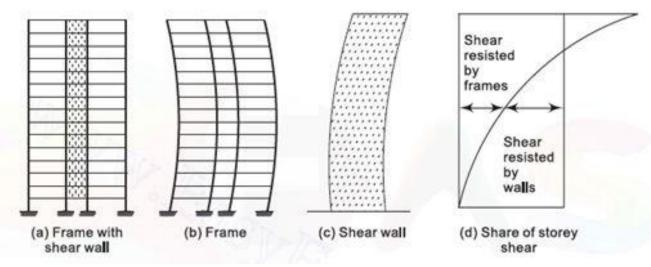
Fig. 2.9 Contribution of frames and shear walls to storey shear (Earthquake Behavior of Buildings, 2012)
