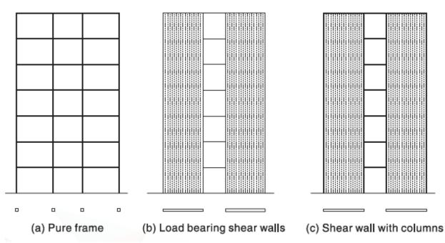
Fig. 2.8 Types of system framing (Earthquake Behavior of Buildings, 2012)
