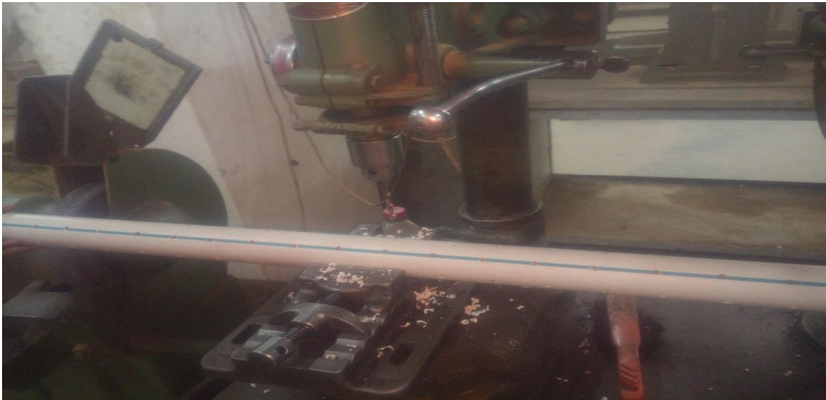
Fig (3.10): Hole process of pipes
