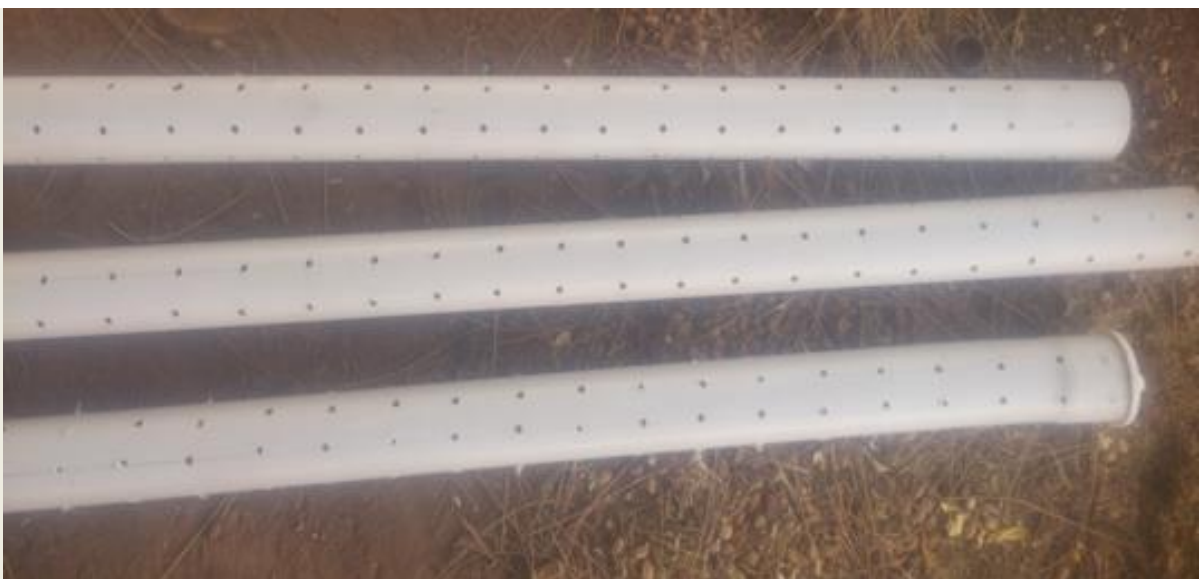
Fig (3.11): The perforated pipes
