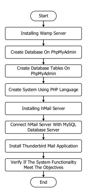
Figure 3.8. Proposed system implementation process flow
