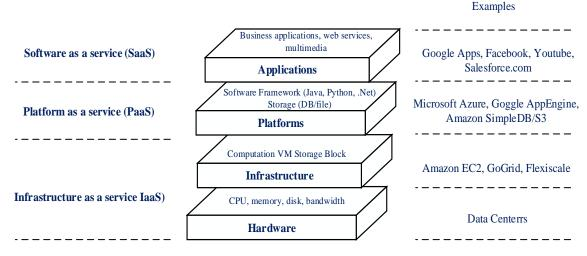
Figure 2.1. Cloud Computing Architecture
