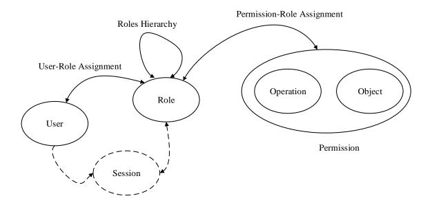
Figure 3.2. Role-based Access Control Model
