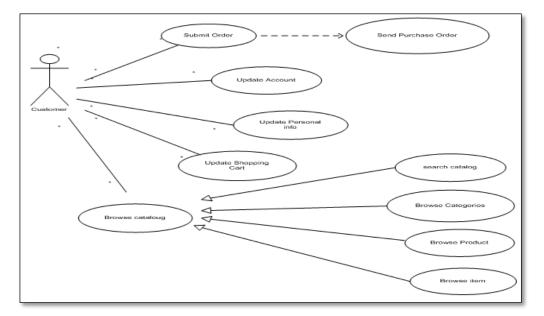
Figure 6.4 Use Case between the Customer and the Web Site.
