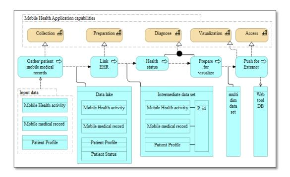
Figure B.7: Mobile Application design and development process.
