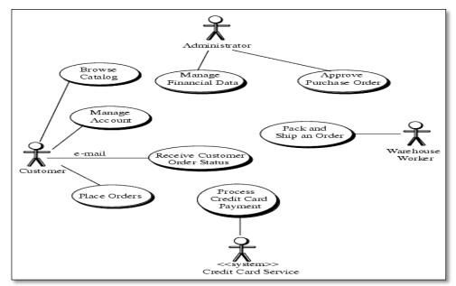
Figure 6.3 Use case diagram for Pet Store Application.
