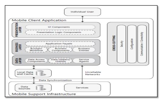
Figure 5.6 Layer Architecture for Mobile Application (Meier et al. 2008).
