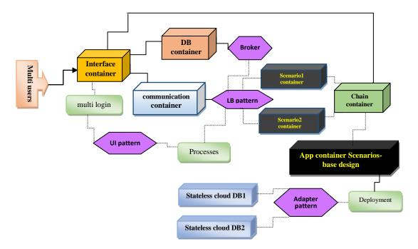
Figure 4.8 An annotated proposed container design for migrating Students Examination Results on clouds.
