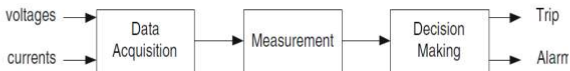
Figure 4.9 Functional Elements of Protective Digital Relay
