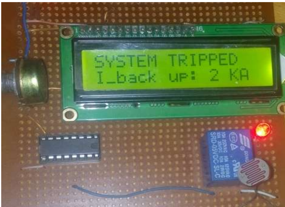
Figure 6.27 Hardware Overcurrent Relay showing the Faulty Operation
