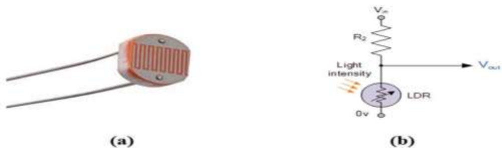
Figure 6.6 Light Dependent Resistor (LDR), (a) Physical view, (b) Wire connection
