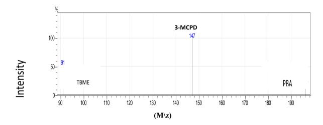
Figure 2 Selective Mass spectrum of (3-MCPD).
