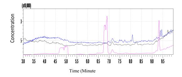
Figure 7 Standards Chromatograms, retention time (min), total areas and concentration of 3-MCPD. 4.1.9 Figure 8 shows calibration curve, the correlation coefficients were (0.9999), with samples having the level of 3-MCPD higher than (1ppm), lower of the sample were used, and relative standard deviation (RSD) were (2.3037).
