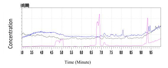
Figure 6 Standards Chromatograms, retention time, (minutes), total areas and concentration of (3-MCPD).
